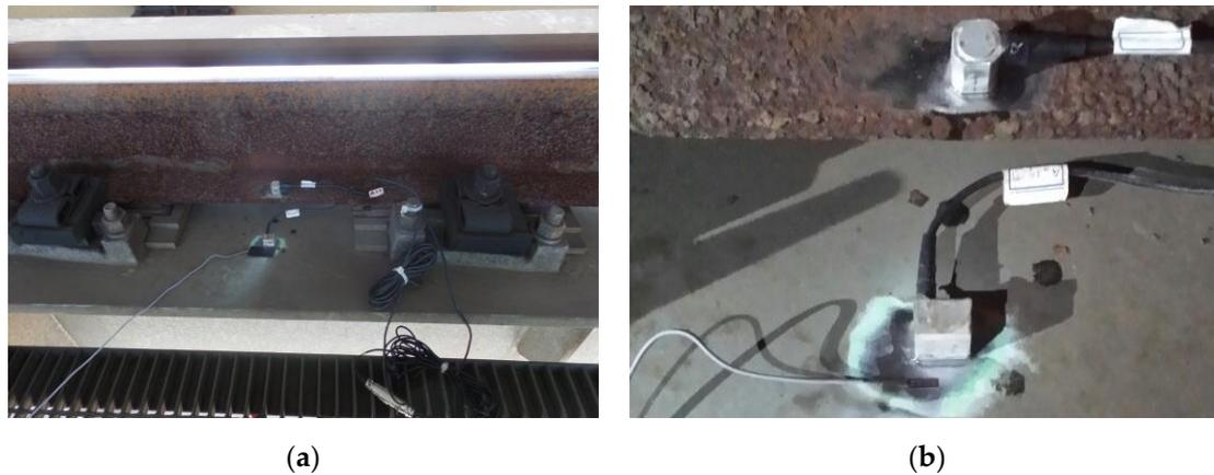
**Figure 11.** Measurement setting for the rail and the track girder: (a) view of accelerometer installation; (b) accelerometer.
