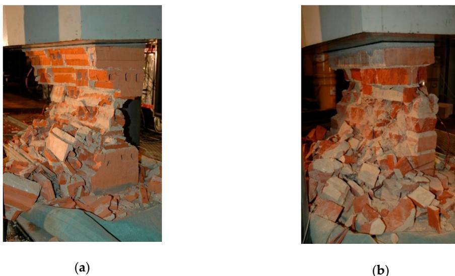
**Figure 10.** Collapse mechanism resulting from compression tests: (a) ceramic hollow brick specimen; (b) ceramic solid brick specimen.
