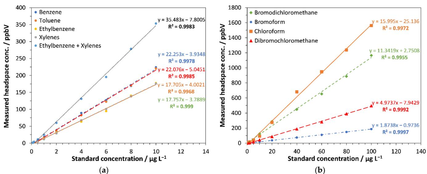
**Figure 2.** Linearity of headspace measurements versus standard concentration averaged across product ions for each compound, showing the linear fit and its regression coefficient,  $R^2$ . (a) BTEX; (b) THMs.
