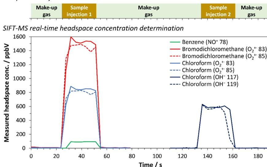
**Figure 1.** Injections for dual sampling of a single vial (calibration levels of 5 and 50  $\mu\text{g L}^{-1}$ , for BTEX and the THMs, respectively), enabling SIFT-MS analysis using both positive (left-hand injection) and negative (right-hand) reagent ions in a single run. Each trace represents real-time measurement of a given quantitation ion, with benzene, bromodichloromethane, and chloroform product ions used as examples.
