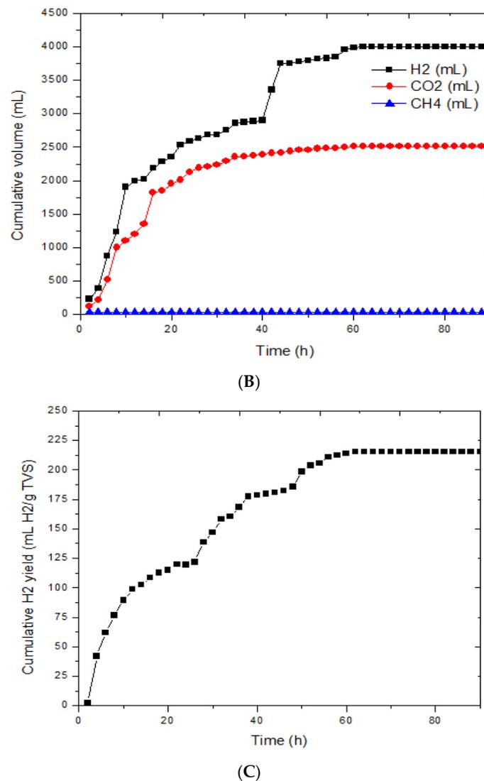
**Figure 1.** (A) Evolution of biogas fraction of hydrogen, methane and carbon dioxide; (B) cumulative biogas volume during biohydrogen fermentation process using immobilized bacteria; and (C) cumulative hydrogen yield.
