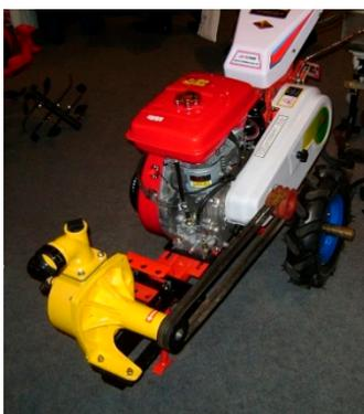
**Figure 7.** Huaxing 2 WT driving a water pump for crop irrigation (Photo: Brian Sims).
