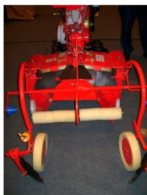
**Figure 6.** Huaxing plastic mulch-laying machine. The tractor forms the 1 m-wide ridge before applying the mulching film (Photo: Brian Sims).
