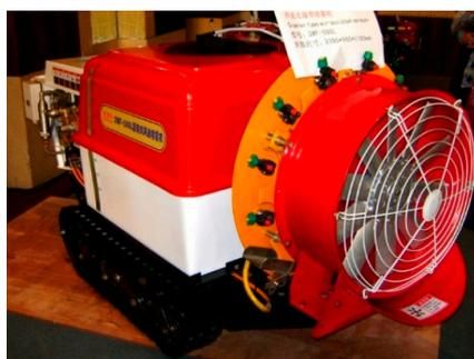
**Figure 13.** Datang hand-operated, or remote-controlled, fan sprayer for tree crops (Photo: Brian Sims).
