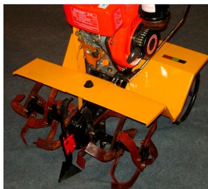
**Figure 4.** Datang 2 WT with rotary cultivator. (Photo: Brian Sims).
