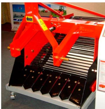
**Figure 10.** Menoble 3-point linkage mounted single row potato harvester for a 30 hp tractor (Photo: Brian Sims).
