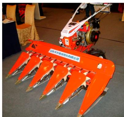
**Figure 5.** Huaxing cereal harvester mounted on a 4 kW (5.4 hp) 2 WT. (Photo: Brian Sims).
