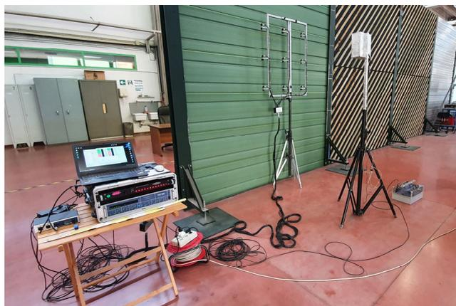
**Figure 1.** Laboratory measurement of sound reflection index according to the EN 1793-5 standard.
