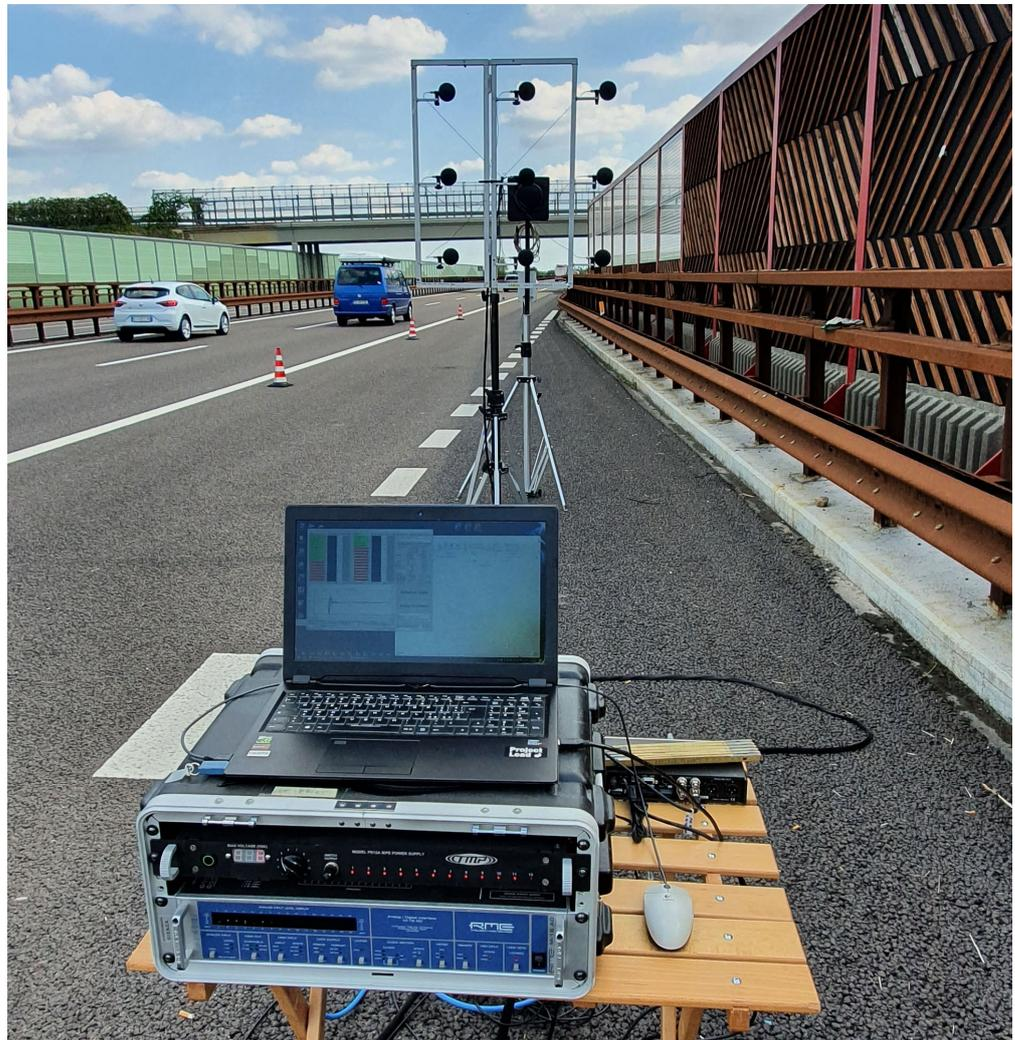
**Figure 4.** In situ measurement of sound reflection index according to the EN 1793-5 standard: free-field measurement (front view) and measurement system.
