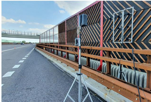
**Figure 2.** In situ measurement of sound reflection index according to the EN 1793-5 standard.
