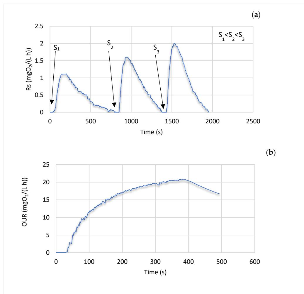
**Figure 2.** Examples of a graph obtained for the evolution of the dynamic rate of oxygen consumption ( $R_s$ ) and a graph obtained for the evolution of the static oxygen uptake rate (OUR). (a) Dynamic test; (b) Static test.  $S_1$ : substrate added 1 (5 mL);  $S_2$ : substrate added 2 (10 mL);  $S_3$ : substrate added 3 (15 mL).
