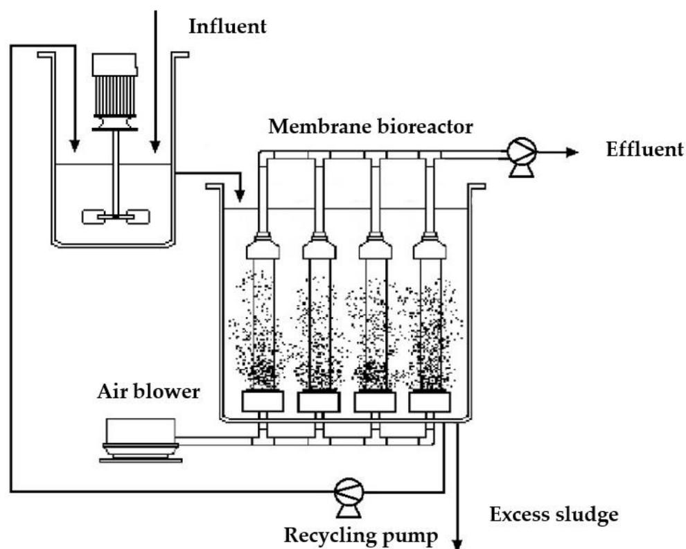
**Figure 1.** Schematic diagram of the pilot plant of an MBR for municipal wastewater treatment used in the study.
