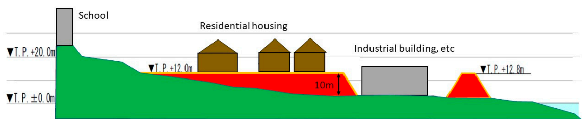
Figure 7. Diagrammatic representation of multi-layer safety interventions at Kirikiri.
