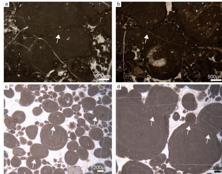
**Figure 5.** Plain polarized light image showing grain contact seams (white arrows) of the grain supported facies in the well-layered unit (a,b) and in the oolitic unit (c,d).
