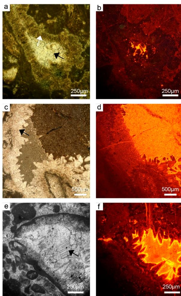
**Figure 9.** (a) Plain polarized light image showing the radial fibrous cements (white arrow) and blocky cements (black arrow). (b) Same image of (a) under CL. (c) Plain polarized light image showing dog-tooth cements (black arrow) and sediment infill. (d) Same image of (c) under CL. (e) Polarized images showing blocky cements (black arrow). (f) Same image of (e) under CL.
