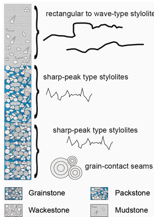
**Figure 11.** Deepening upward cycle characterizing the facies stacking of the well-layered unit in the SLM site. On the right side is the classification of stylolites in relationship to the facies textures.
