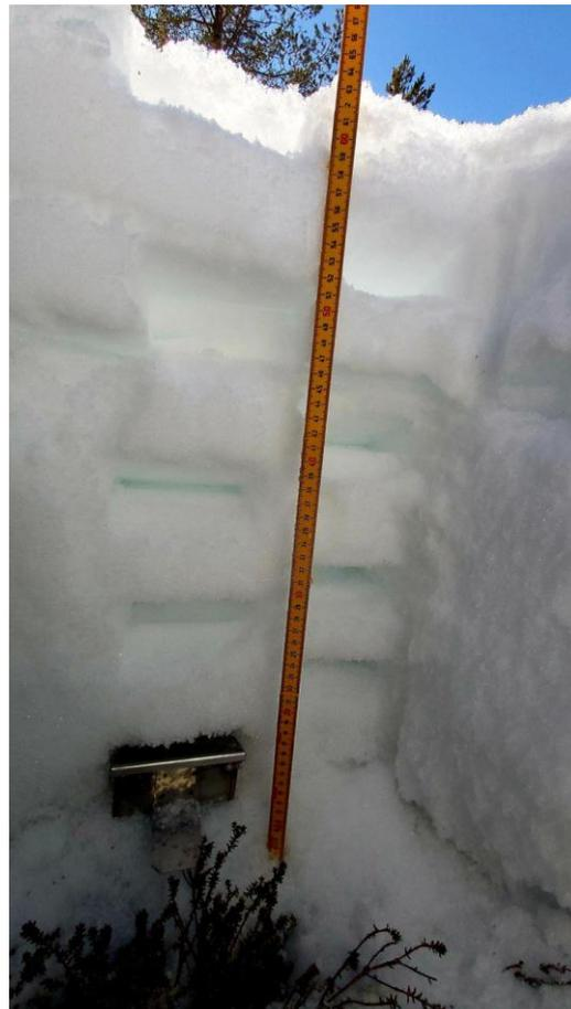
**Figure 3.** The density profile was measured using a 250 cm<sup>3</sup> RIP2 density cutter.
