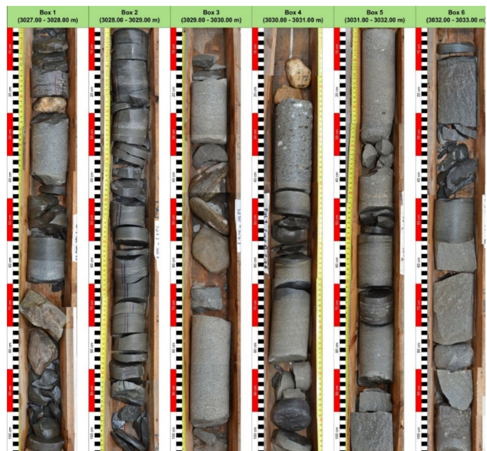
Figure 6. Core photographs of PO-1 illustrating sedimentological characteristics of the deepwater facies association. The sandstone beds are often structureless and display sharp and often erosional bases with the underlying deposits. Occasionally, sandstones are overlain by finer-grained mudstone and suggest a general fining upward trend.
