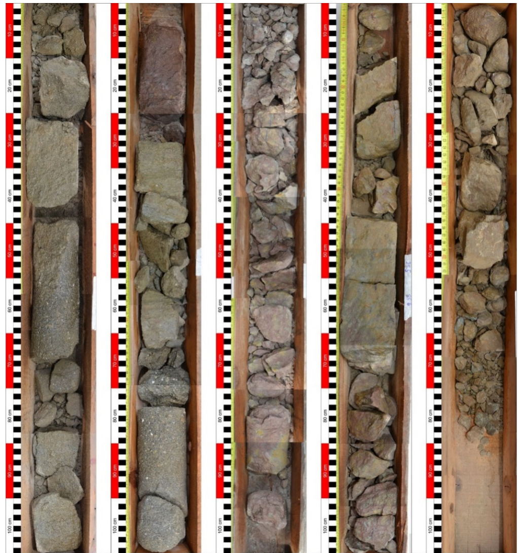
Figure 4. Core photographs of PO-1 illustrating sedimentological characteristics of the fluvial facies association. Coarser-grained sedimentary rocks that belong to fluvial channels (Fl.ch) overlay finer-grained deposits of the overbank facies (Fl.v).
