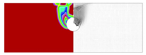
**Figure 9.** Shear strain rate (SSR) and velocity plot for C/D = 1,  $\gamma D/S_u = 1$ .
