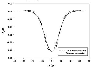
Figure 13. A typical regression of the Gaussian equation to the FLAC data.
