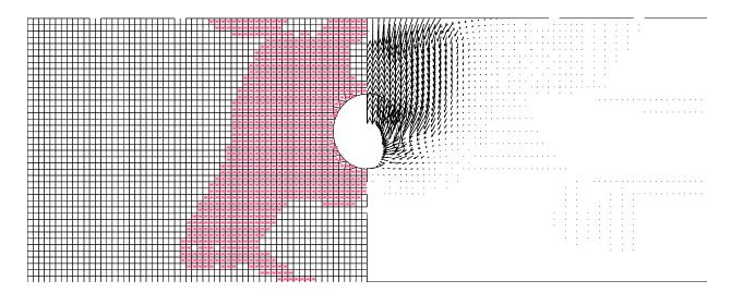
**Figure 6.** Plasticity (left), and velocity (right) plots at the stage of collapse (C/D = 1,  $\gamma D/S_u = 3$ ).
