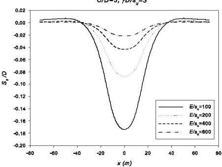
**Figure 16.** Typical settlement profiles with respect to  $E/S_u$  (Young's modulus ratio).
