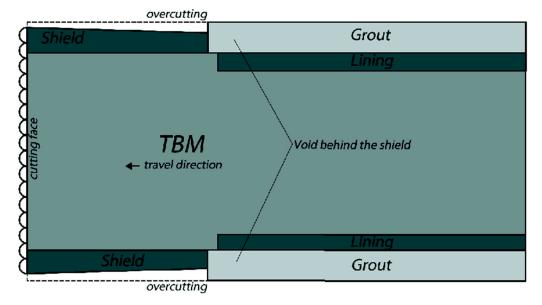
Figure 1. Schematic diagram of a TBM indicating overcutting (not to scale).
