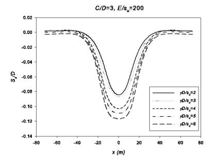
**Figure 15.** Typical settlement profiles with respect to  $\gamma D/S_u$  (soil strength ratio).
