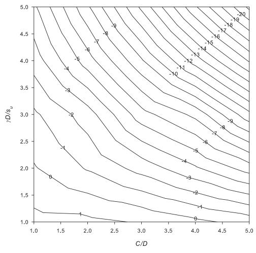
**Figure 8.** Contour plot of critical stability numbers,  $N = (\sigma_s - \sigma_t)/S_u$ , obtained from this study.
