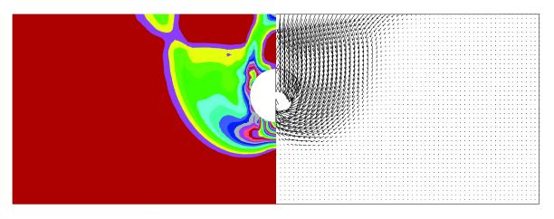
**Figure 10.** Shear strain rate (SSR) and velocity plot for C/D = 1,  $\gamma D/S_u = 5$ .
