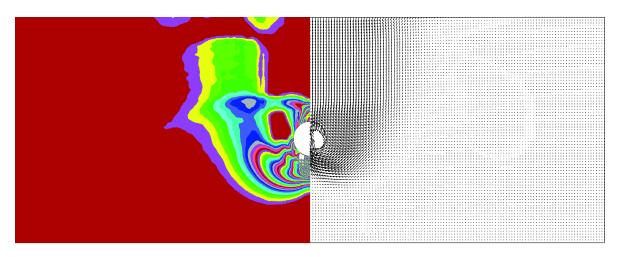
**Figure 12.** Shear strain rate (SSR) and velocity plot for C/D = 3,  $\gamma D/S_u = 5$ .
