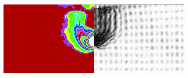
**Figure 11.** Shear strain rate (SSR) and velocity plot for C/D = 3,  $\gamma D/S_u = 1$ .
