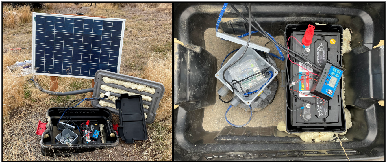
Figure 4. Seismic station composed of the buried, sealable container with solar panel and an inner view of the container with the marine battery and weatherproof case containing the seismometer.
