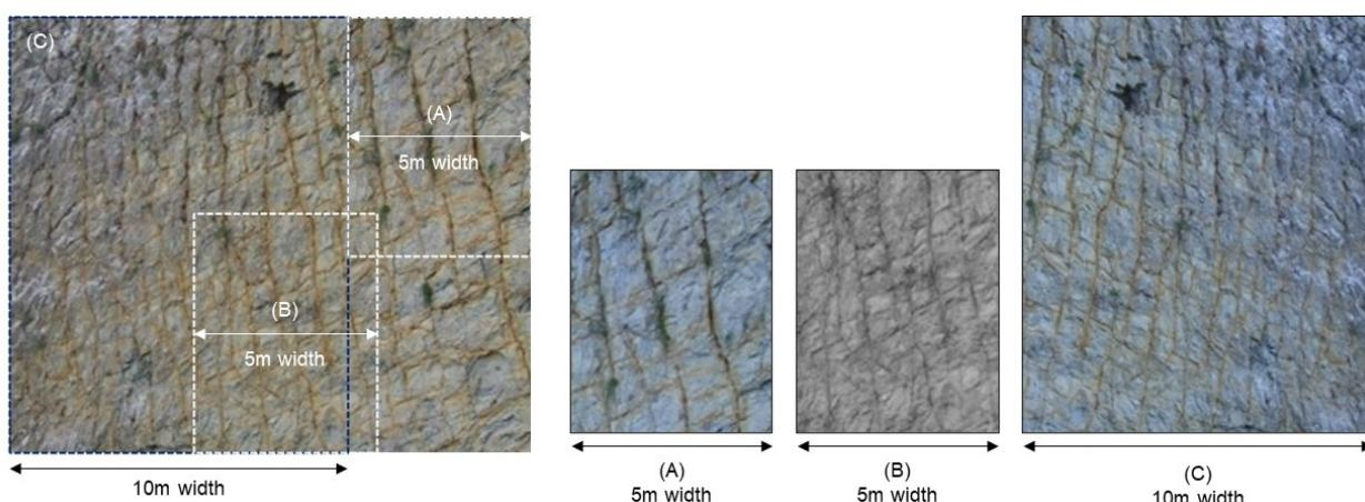
**Figure 9.** Outcrop used as part of the survey described in the text to analyse the subjectivity of the processes by which different persons would determine GSI.
