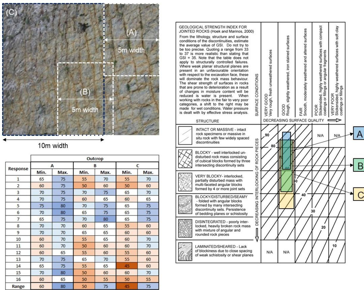
**Figure 10.** Results of the survey analysing the subjectivity of the processes by which different persons would determine the GSI of the three—only apparently different—rock outcrops.
