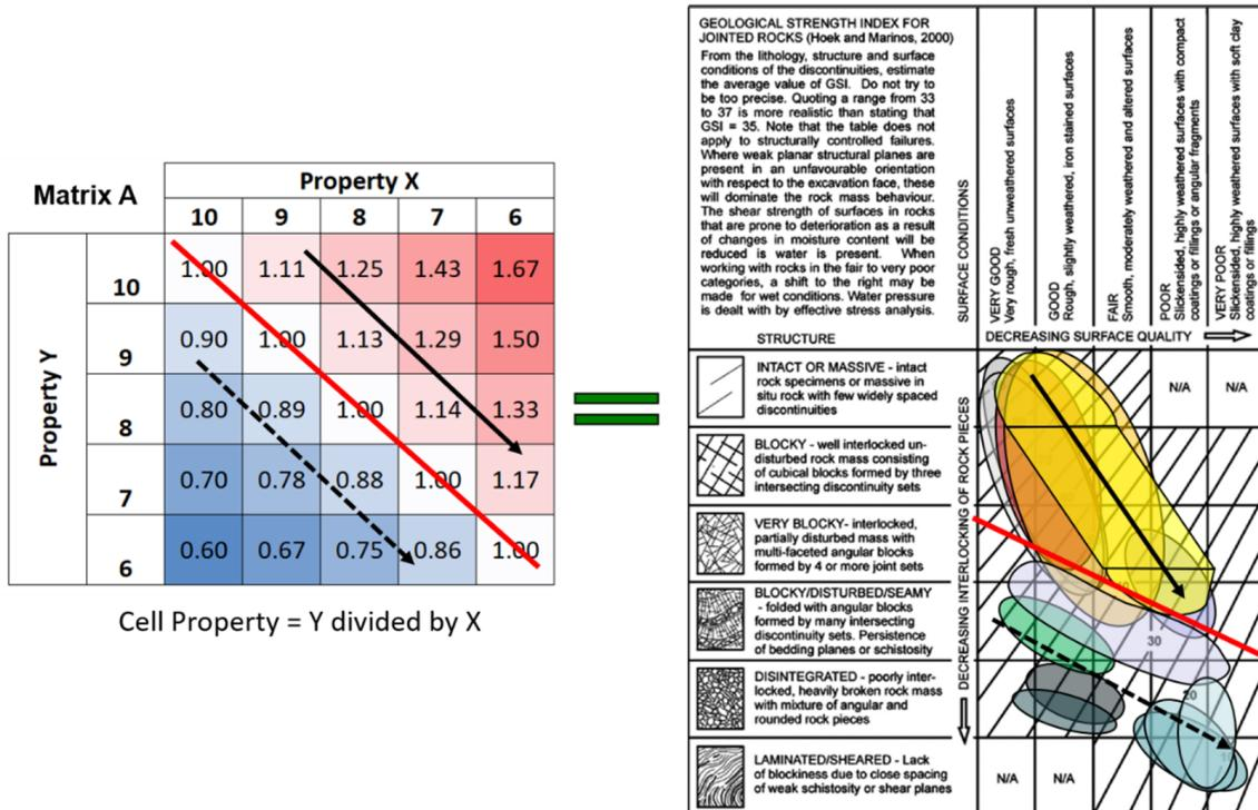
Figure 8. Comparison between Matrix A and the GSI system [45] when new (geological) knowledge is included.
