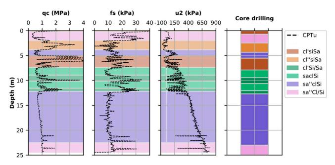
Figure 2. Example of the assignment of core drillings to CPT-data by Oberhollenzer et al. [8].
