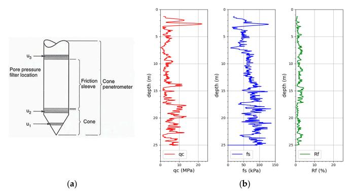
**Figure 1.** (a) Scheme of the CPT probe, which is pushed into the subsoil [17]. (b) Example of measured data from the cone penetration test (cone resistance  $q_c$ , sleeve friction  $f_s$  and the friction ratio  $R_f$ ).
