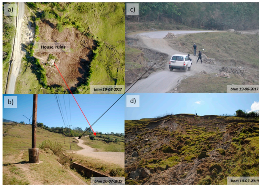
Figure 6. Evidence of ground deformation and its impact: (a) house ruins, (b) electrical pole that moved and tilted, (c) degraded road conditions, and (d) small landslide induced by an earthquake.
