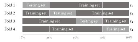
**Figure 3.** Four-fold Cross-Validation. The original dataset is partitioned into 4 equally sized subsets, which are repeatedly used as either test or training sets.
