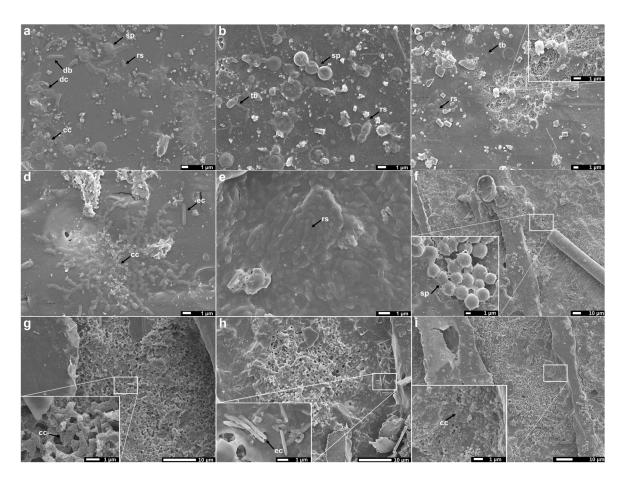
**Figure 2.** Scanning electron microscopy images of PLA (**a**–**c**) and PHBV (**d**–**i**) films exposed to a marine environment for 6 months. Arrows indicate identified microbial structures. cc: Coccoid cell; db: diplobacilli; ec: elongated cell; rs: rod shape; sp: sporous; tb: tubular.
