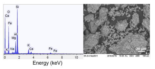
Figure 2. SEM Image and EDS Analysis of Raw Zeolite Particle.
