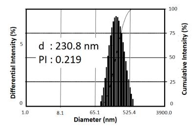
Figure 3. Particle Size Analysis of ZNPs Suspension.
