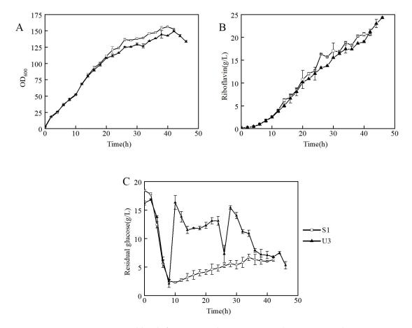
**Figure 3.** Fed-batch fermentation by strains S1 and U3 in a 7.5-L bioreactor containing 3 L of fermentation medium. (**A**) time course profile of cell growth; (**B**) riboflavin production during fermentation; (**C**) concentration of residual glucose.
