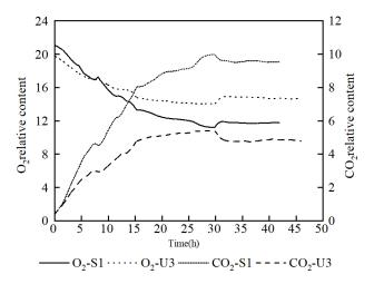
Figure 4. Comparison of off-gas analysis data between S1 and U3 on fed-batch fermentation.
