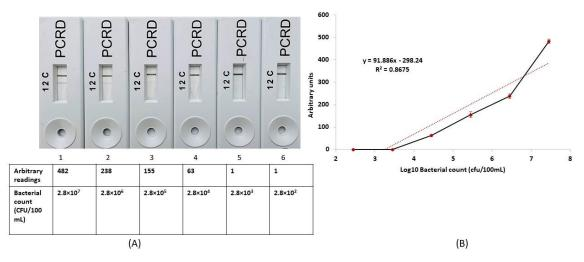
**Figure 6.** (**A**) Comparison of the RPA-LFA visual outputs and the values recorded by the GT810. (**B**) Standard curve plot of bacterial cell numbers v GT810 readings; (•) represents the value produced by the LF reads corresponding to the CFU count of bacteria per 100 mL of growth medium.
