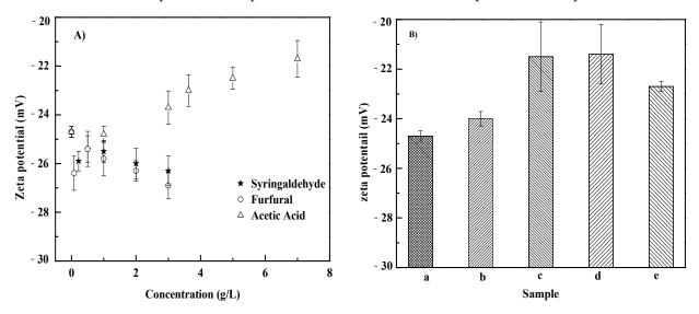
**Figure 3.** Effects of inhibitors on zeta potential at 72 h. (**A**) Individual inhibitor group; (**B**) Inhibitor cocktails. a–e represent the group of blank, cocktail of 3.63 g/L acetic acid + 0.22 g/L furfural, 3.63 g/L acetic acid + 0.08 g/L syringaldehyde, 0.22 g/L furfural + 0.08 g/L syringaldehyde, and 3.63 g/L acetic acid + 0.22 g/L furfural + 0.08 g/L syringaldehyde, respectively.
