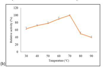
**Figure 5.** Temperature optimum and stability of the purified *A. geothermalis* ALDH. (a) Effect of temperature on the activity of aldehyde dehydrogenase. (b) Effect of temperature on the stability of aldehyde dehydrogenase.
