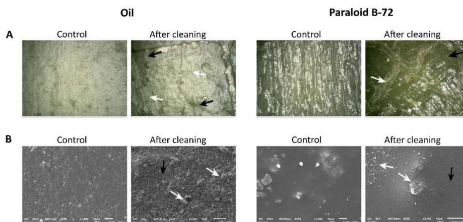
**Figure 10.** The efficacy of esterase-based cleaning treatments on murals (painted laboratory models) covered by sunflower oil or Paraloid B-72, evaluated by optical microscopy (A) and SEM (B). The white arrows indicate the cleaned areas, while the black arrows indicate the areas where the targeted substrates were not removed due to the uneven distribution of the enzyme on samples' surfaces.
