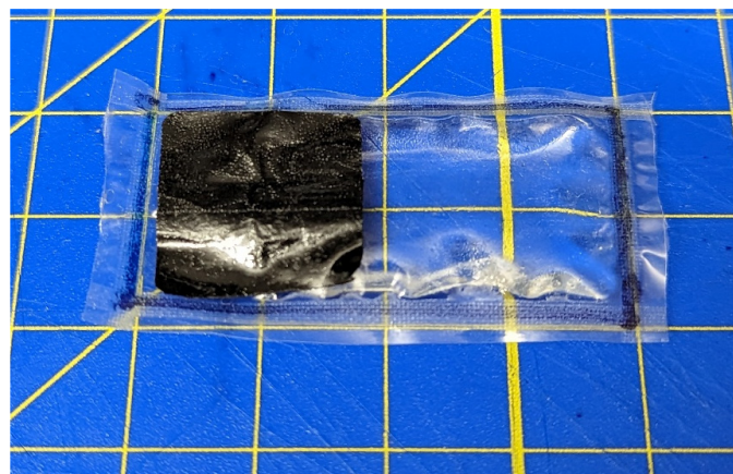
Figure 1. Example of a HASEL actuator created in the lab. The actuator pictured has a carbon tape electrode, a low-density polyethylene shell, and is filled with mineral oil.
