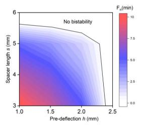
**Figure 6.** The combined effects of spacer length s and pre-deflection h on the minimum net-force  $F_n(\min)$  of the bistable SMA actuator. The limit of bistability is reached when  $F_n(\min)$  becomes zero, as indicated by the solid line.
