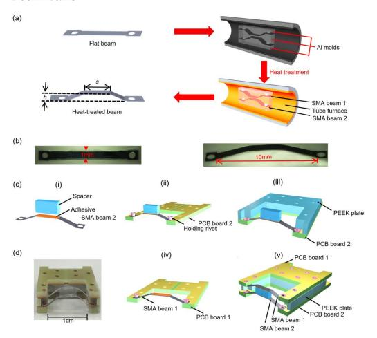
**Figure 3.** Shape-setting and assembly process of the bistable actuator. (a) Schematic of heat treatment in a vacuum tube furnace; (b) photos of the SMA beam before and after heat treatment; (c) schematic assembly process; (d) photo of the bistable SMA actuator. Heat sources 1 and 2 are not shown for clarity. Legend: s—spacer length, h—pre-deflection.
