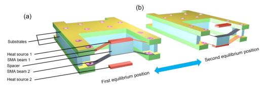
**Figure 2.** Layout of the bistable SMA actuator. At sufficiently high temperature of the heat sources 1 and 2 an oscillatory motion occurs between the two equilibrium positions shown in (**a**,**b**).
