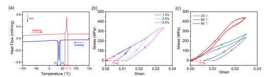
**Figure 1.** (a) Differential scanning calorimetry (DSC) measurement of a TiNiCu film of 15  $\mu$ m thickness; (b) stress–strain characteristics of a TiNiCu tensile test specimen at different maximum strain in the range of from 1.5 to 3.5% at a low strain rate of  $10^{-3}/s$  at room temperature; (c) stress–strain characteristics of a TiNiCu tensile test specimen at different temperatures in the range of from 23 to 80 °C at a strain rate of  $10^{-3}/s$ .
