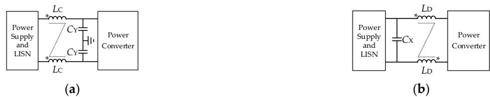
Figure 12. Basic structures of passive EMI filters. (a) CM filter; (b) DM filter.
