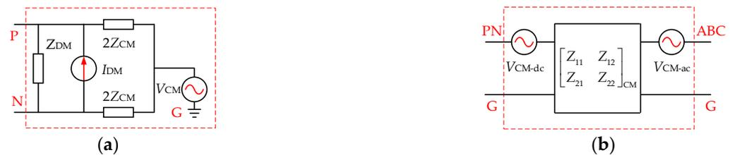
**Figure 6.** Behavioral models for motor drive systems. (a) Three-terminated network [63]; (b) two-port unterminated network [64].
