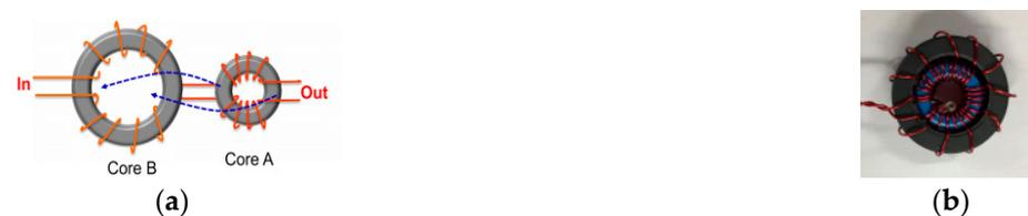
**Figure 14.** Novel CM inductor with reduced near-field coupling [89]. (a) Winding connection; (b) prototype.
