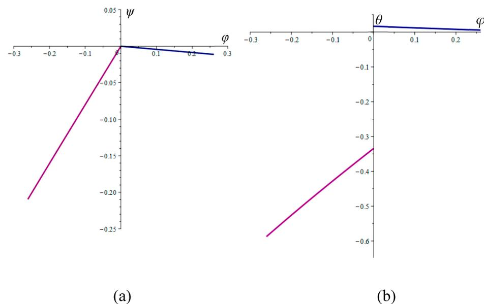
**Figure 9.** The output parameters of the involute cam: (a) The position output angle  $\psi$  [rad]; (b) The pressure angle  $\theta$  [rad].
