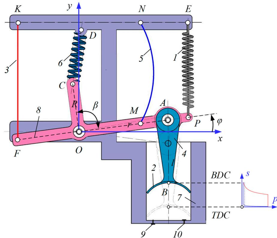
**Figure 1.** Kinematic scheme of the bistable pump with recuperative springs [32,33]: 1. Piston spring; 2. Piston; 3. Discharge SMA wire; 4. Coupler; 5. Suction SMA wire; 6. Recuperative spring; 7. Piston cylinder; 8. Three-arm rocker; 9. Discharge valve; 10. Suction valve.
