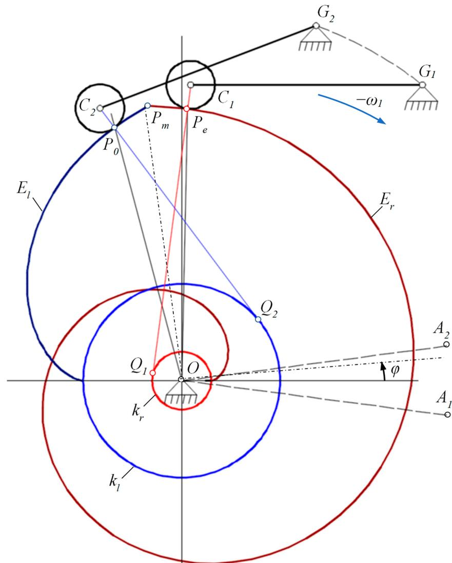
**Figure 6.** Profile of the two-section involute cam.
