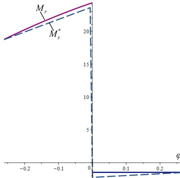
**Figure 10.** The graph of the synthesized recuperative moment  $M_r$  compared to the reference recuperative moment  $M_r^*$ .
