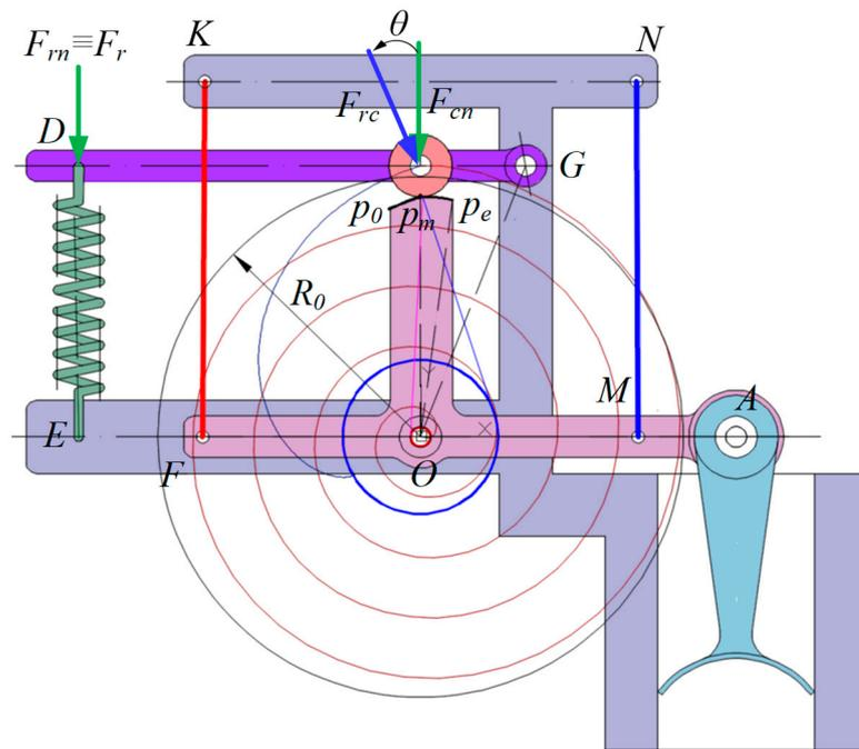
**Figure 8.** Schematic diagram of the pump bistable mechanism with two-section involute cam and oscillating follower in horizontal position of the rocker’s arm OA.
