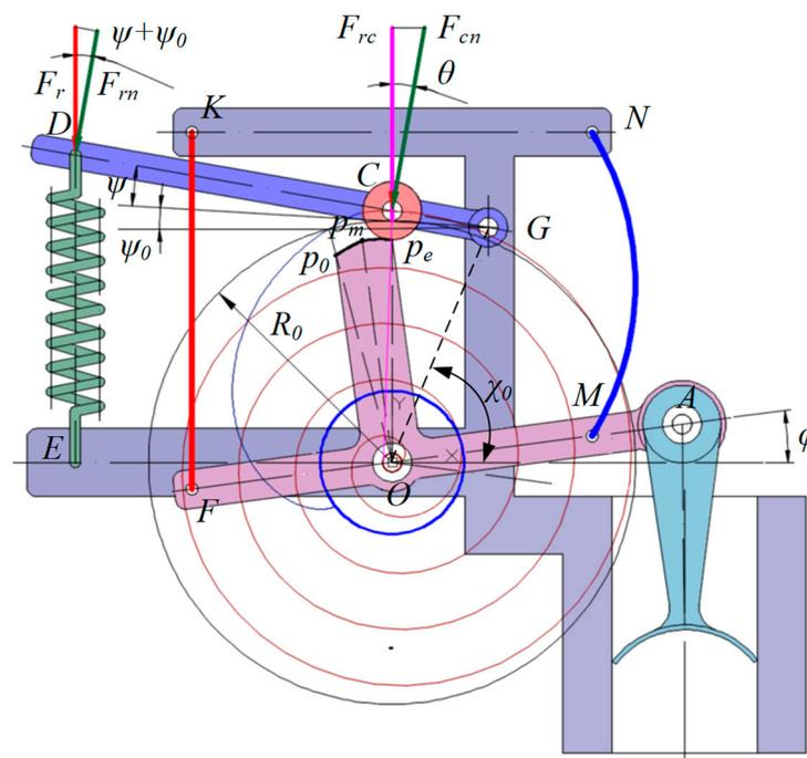
**Figure 7.** Schematic diagram of the bistable pump with two-section involute cam and oscillating follower.
