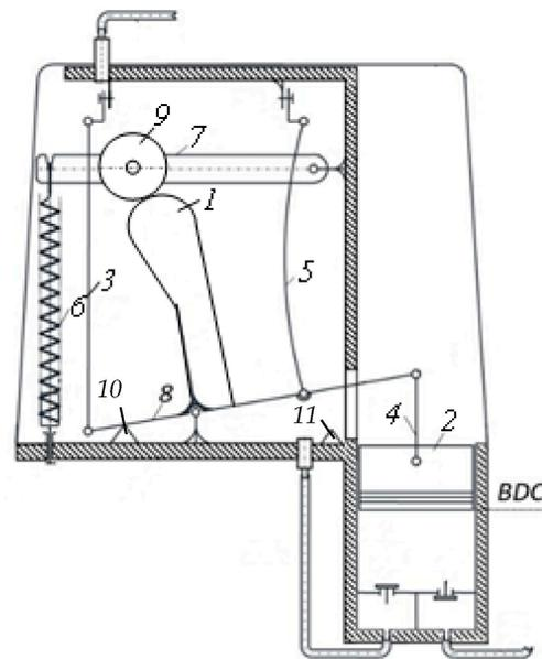
**Figure 5.** Scheme of a pump with a recuperative cam mechanism: 1. Cam; 2. Piston; 3. Discharge SMA wire; 4. Coupler; 5. Suction SMA wire; 6. Recuperative spring; 7. Oscillating follower; 8. Three-arm rocker; 9. Roller; 10. Left end stop; 11. Right end stop.
