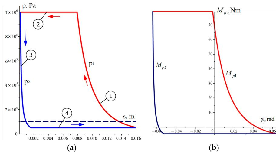
**Figure 2.** Indicator diagram: (a) In pressure-displacement coordinates  $p$ - $s$  [32]; (b) In coordinates moment-angle of rocker arm  $M_p$ - $\varphi$ .
