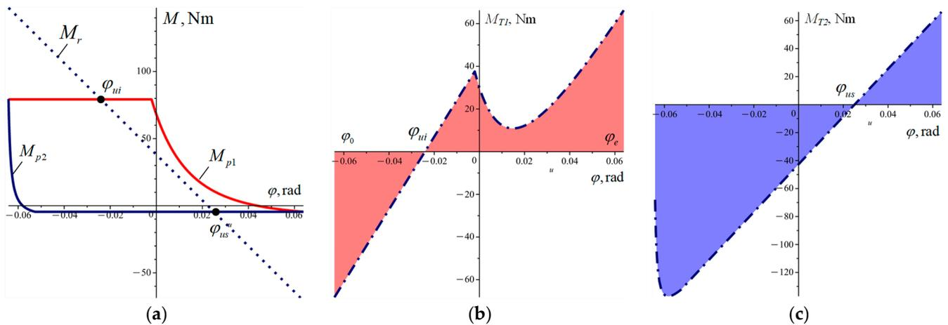
**Figure 3.** Recuperation by a spring with a linear characteristic: (a) View of the linear characteristic and indicator diagram; (b) Resultant moment for the discharge period after the recuperation; (c) Resulting moment for the suction period after the recuperation.
