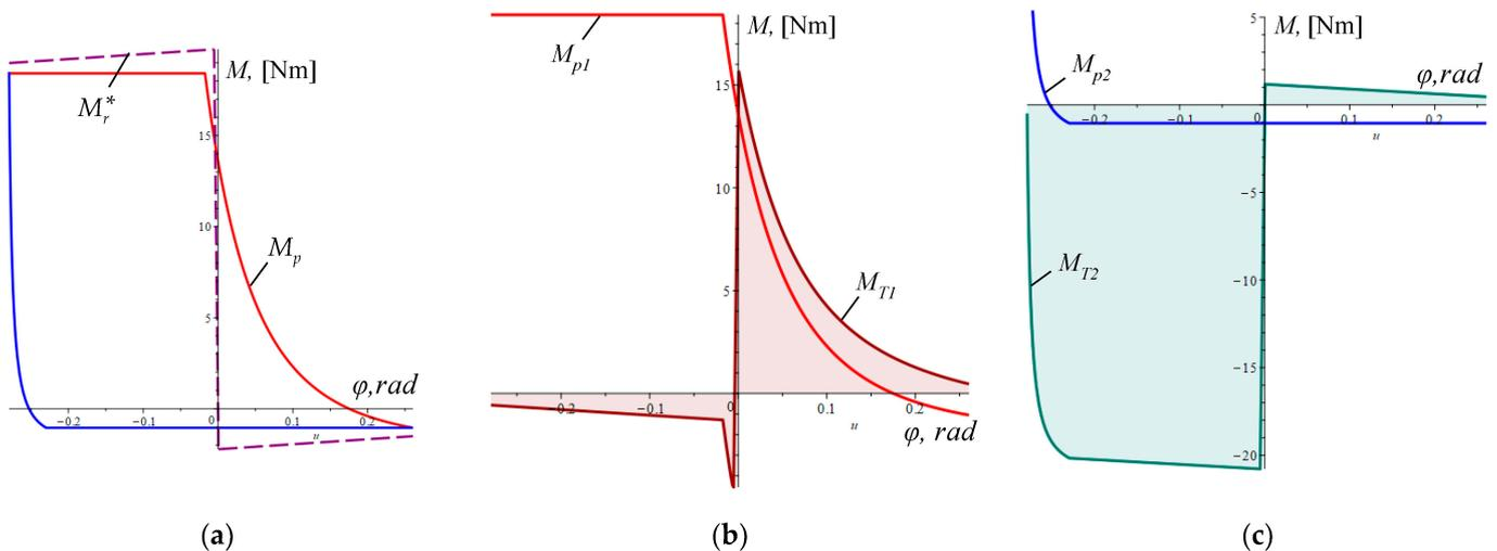
**Figure 4.** Influence of the recuperative moment on work distribution (shaded areas): (a) Indicator diagram and the reference recuperative moment; (b) Work of the reference recuperative moment and piston moment at discharge period; (c) Work of the reference recuperative moment and piston moment at suction period.
