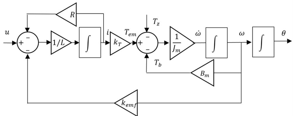
Figure 2. Electrical DC motor complete block diagram.
