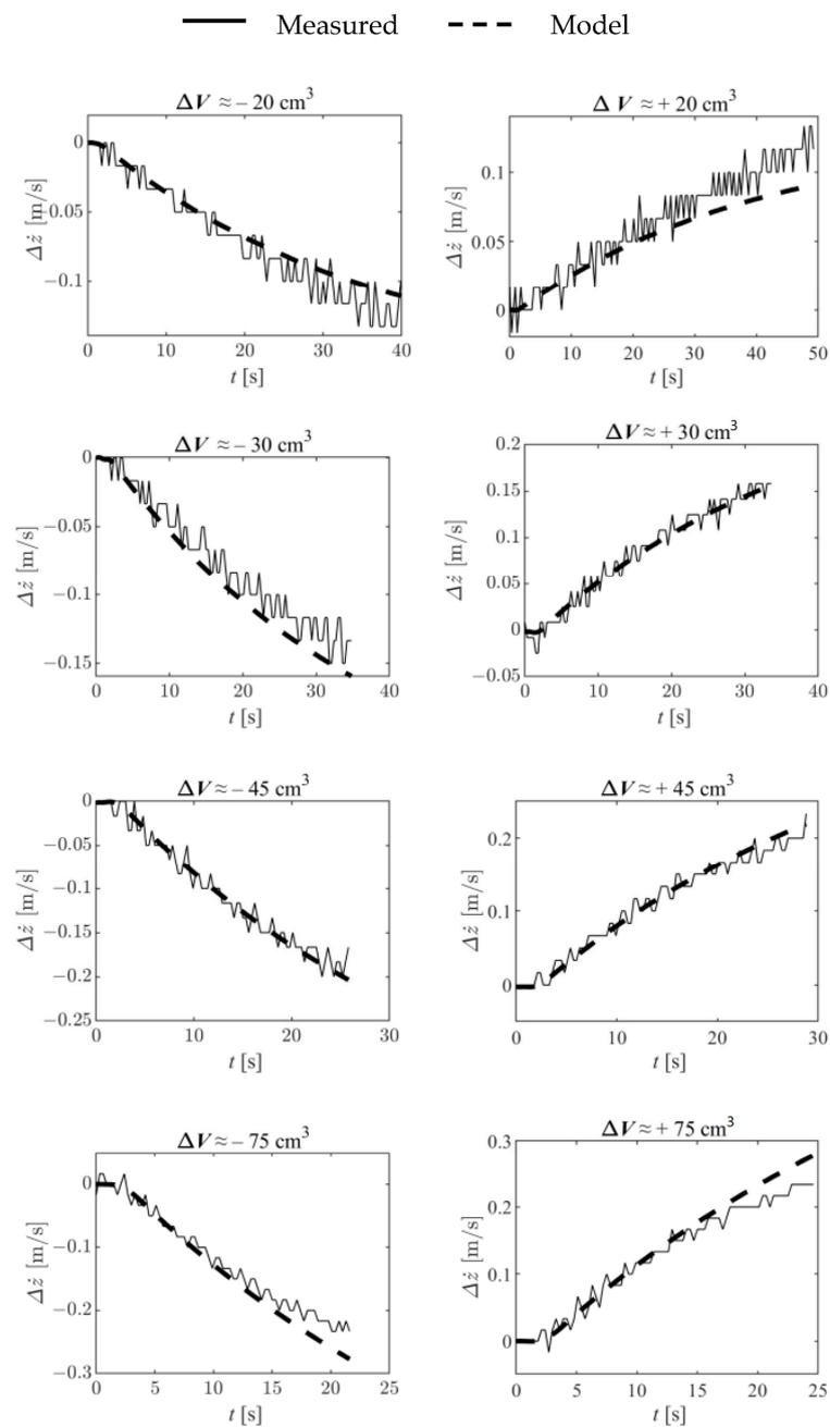
**Figure 13.** Depth velocity identification results: depth velocity evolution in time for different buoyancy changes.
