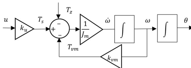
Figure 3. Electrical motor simplified block diagram.
