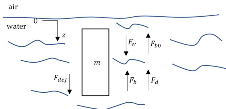
**Figure 9.** Schematic of the forces acting on the VBS device.
