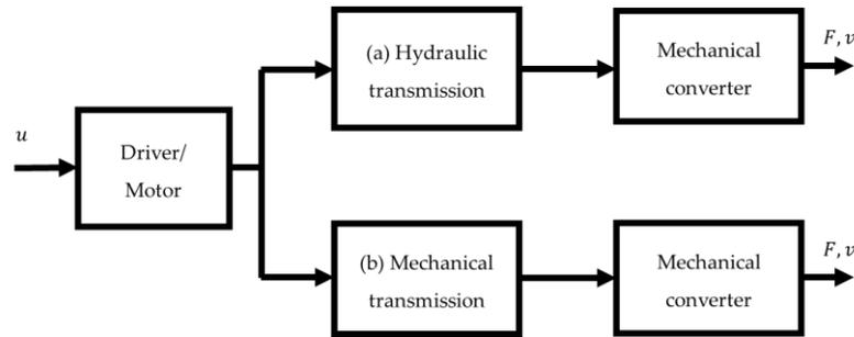
Figure 1. Generic diagram of the actuator elements in a VBS.
