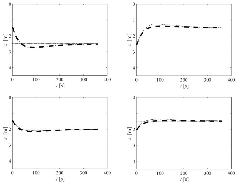
Figure 16. Control results for depth steps of different amplitudes and directions.
