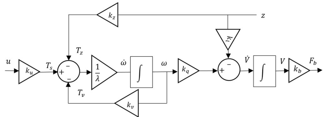
Figure 8. Simplified unified block diagram for the actuation system of the VBS.
