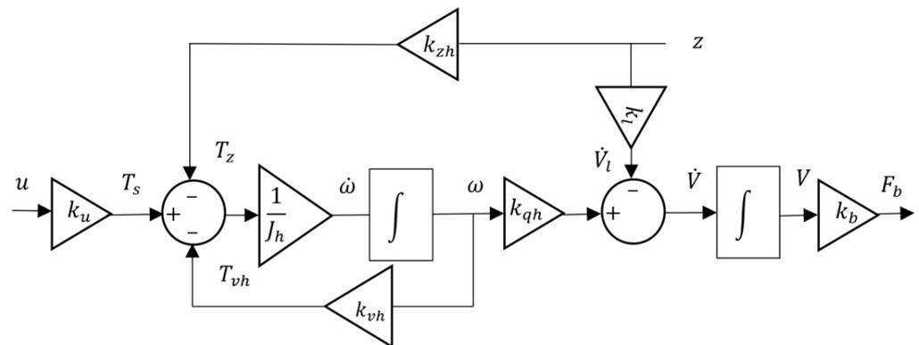
Figure 5. Simplified block diagram of the electrohydraulic solution.
