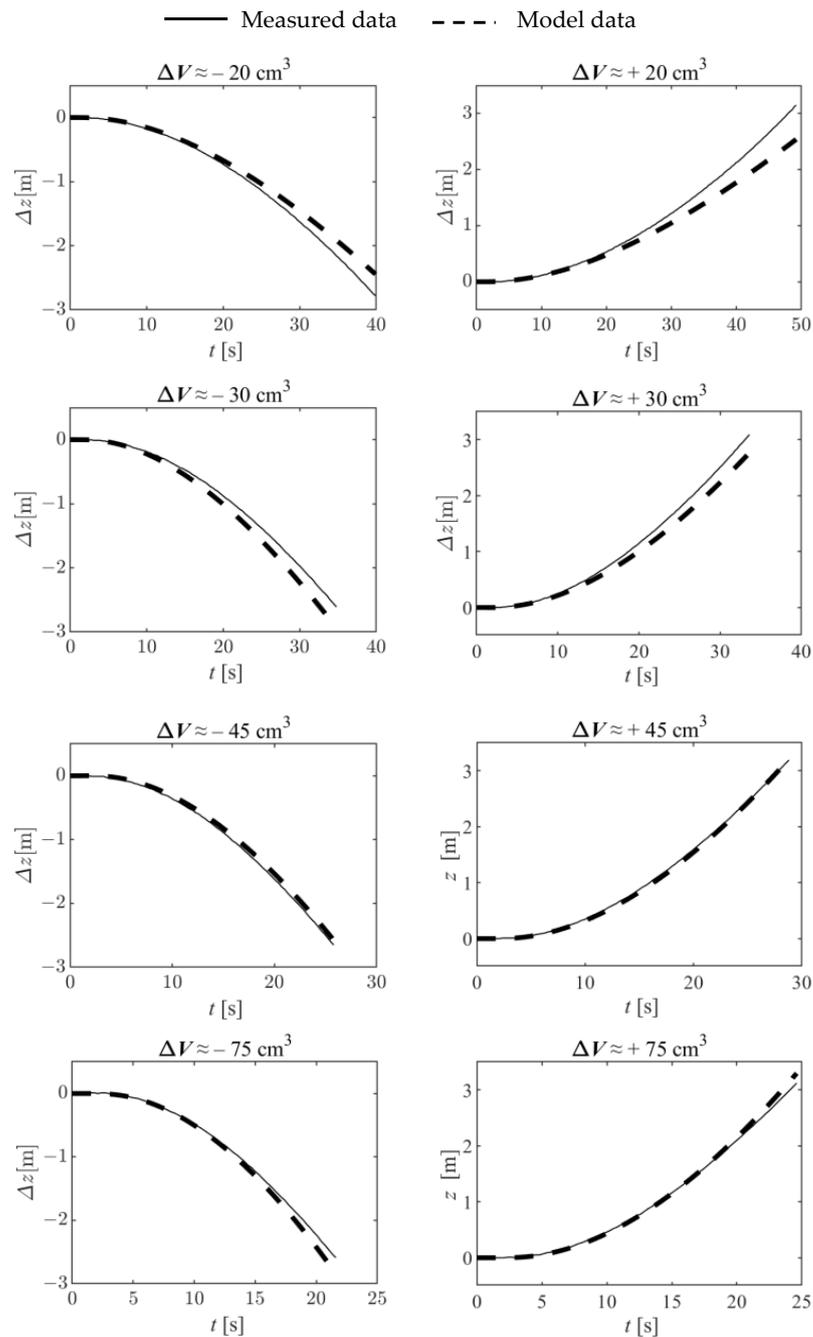
**Figure 14.** Depth identification results: depth evolution in time for different buoyancy changes.
