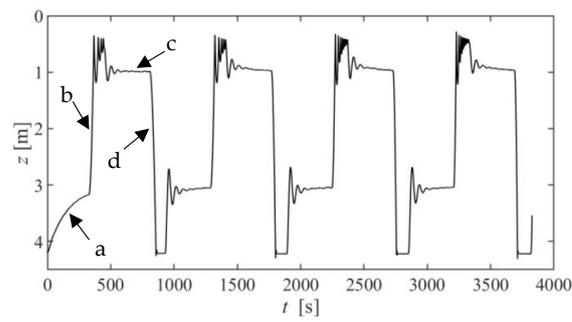
**Figure 12.** Evolution of depth ( $z$ ) in time for the 4 steps of the experimental model identification procedure (a) to (d).
