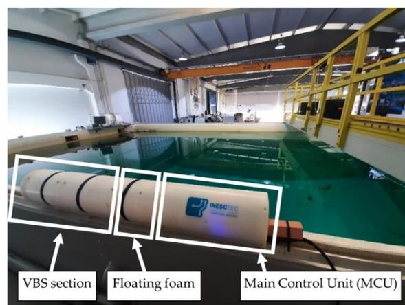
**Figure 11.** Prototype used for model identification and control at the test pool.
