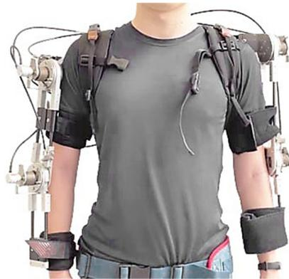
**Figure 2.** Photograph of the upper-limb exoskeleton power assist system.
