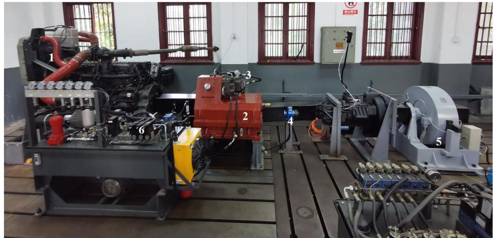
**Figure 5.** Test bench to verify the simulation test platform based on SimulationX. It includes the: ① engine, ② transmission assembly, ③ pump–motor system, ④ rotating speed–torque sensor, ⑤ electric eddy current dynamometer, and ⑥ hydraulic control system.
