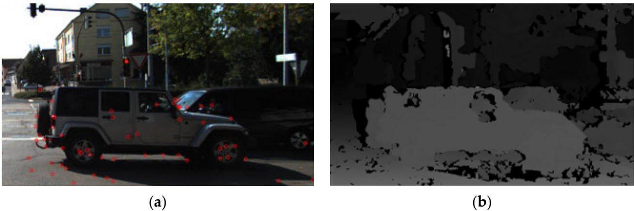
**Figure 4.** The disparity image obtained by LRBM. (a) Original image with feature points, (b) computed disparity image.
