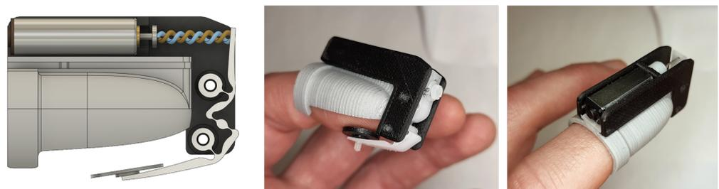
**Figure 9.** CAD of the internal components of the final design, and pictures of the implemented prototype, evidencing the slim design of the main body (black plastic) and the interchangeable soft thimble (light gray polymer).
