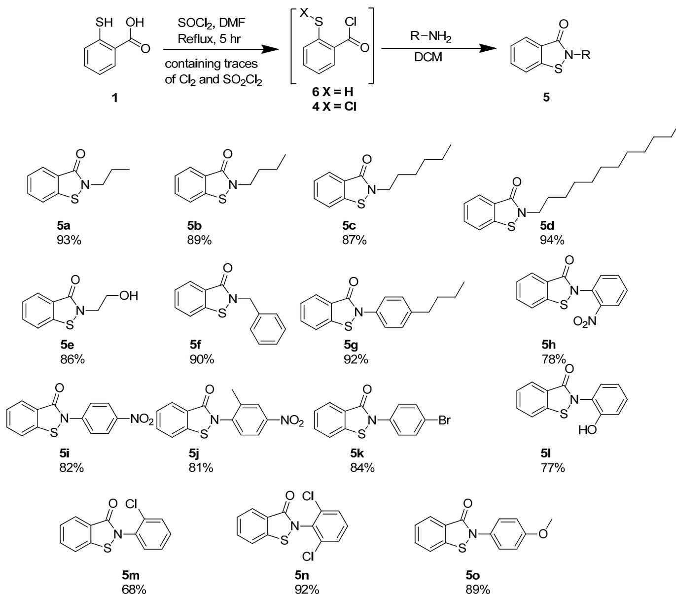
**Scheme 3.** Synthesis of the *N*-substituted BITs with their associated yields.
