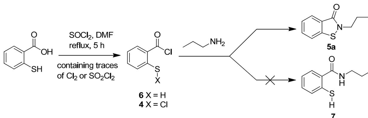
**Scheme 2.** Two-step, one-pot synthesis of BIT **5a** depicting the proposed formation of 2-chlorosulfonyl benzoylchloride (**4**) as an intermediate.
