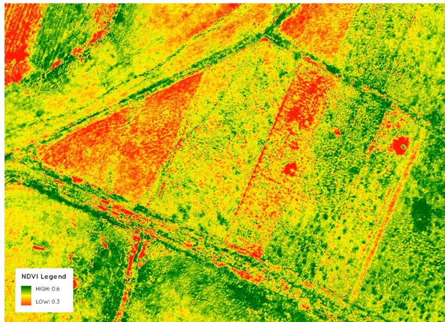
**Figure 7.** NDVI index used to identify areas with more or less vegetation. The red pixels identify soil that is not covered by crops or vegetation. (Source: <https://www.precisionhawk.com> accessed on 29 June 2023).
