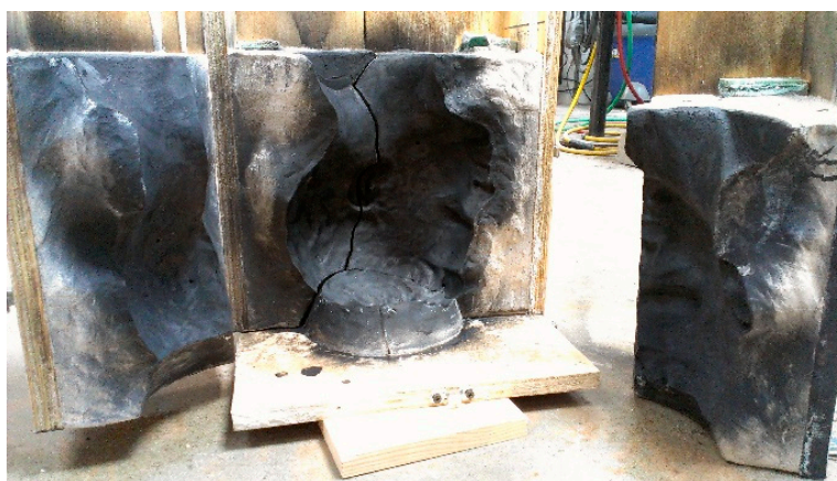
Figure 6. Hinged, 5-part plaster blow mold coated with graphite in preparation for hot glass. [Created by author].
