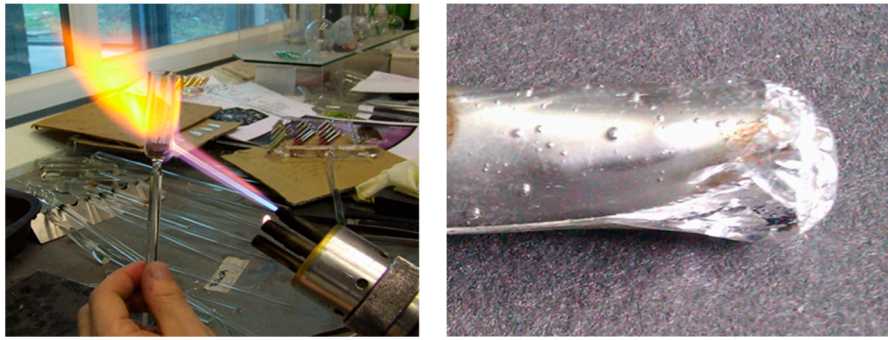
Figure 6. Gallium inclusion applied in borosilicate glass by lampworking; created by author.
