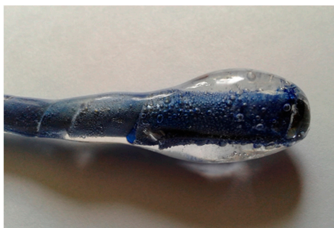
Figure 5. Kovar inclusion applied in borosilicate glass by lampworking; created by author.
