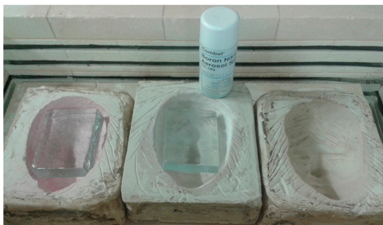
Figure 11. Three types of separators: boron nitride, a slab of cast glass from furnace, and only 1% kiln wash, and/or China clay in the mold mixture; created by author.
