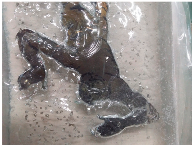
Figure 7. The metal/glass bond caused stress during the cooling process; created by author.
