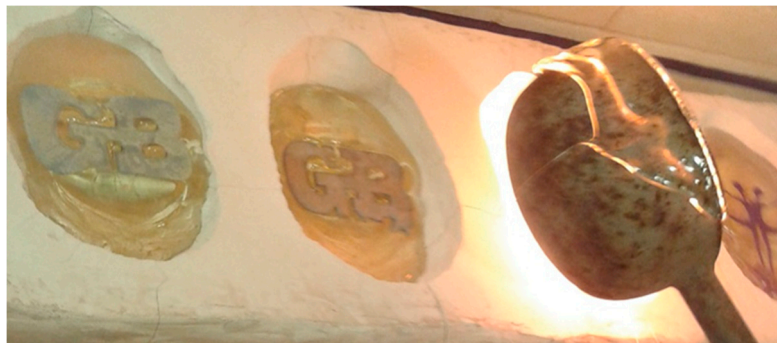
Figure 10. Method of pouring hot glass into plaster molds. The high temperature resistant moulds, up to 900 °C; created by author.
