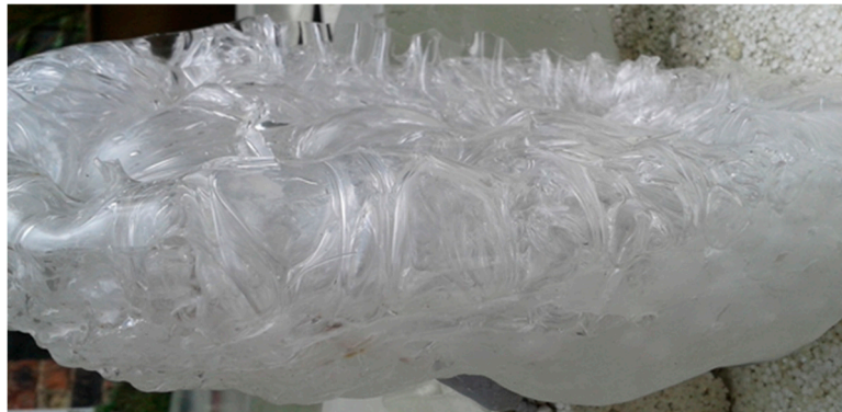
Figure 12. Gas bubbles in the glass as a result of pouring hot glass into the plaster mold; created by author.
