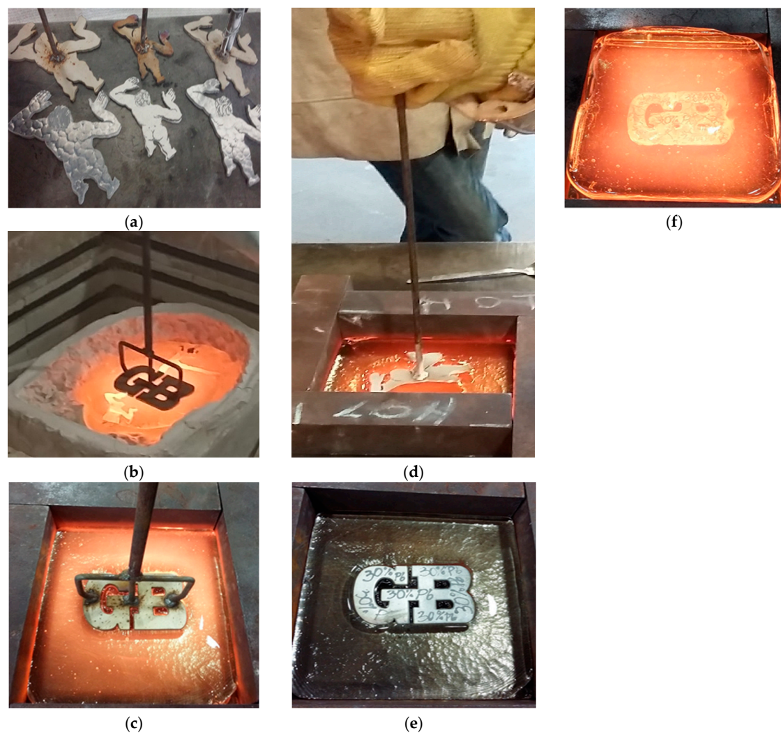
Figure 13. Stamps to make indentations in hot glass and application of lead and tin alloy inclusions: (a) Three sizes of nickel alloy stamps and lead and tin alloy inclusions exactly in the shape of the stamps; (b,c) indentation made by a stamp in the GB shape; (d) indentation made by a stamp in a man silhouette shape; (e) application of lead and tin alloy inclusion; (f) lead and tin alloy inclusion covered by second layer of hot glass; created by author.
