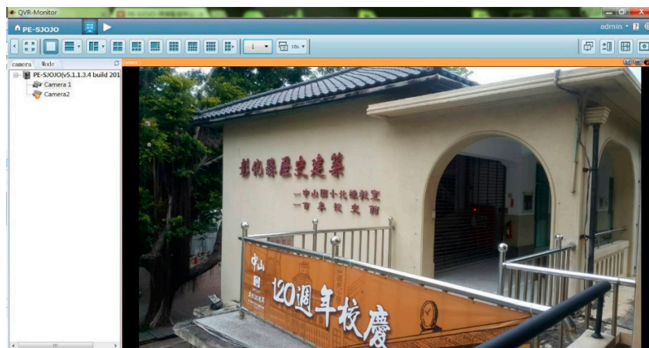
Figure 8. Backup interface of the surveillance and management system on a personal computer.
