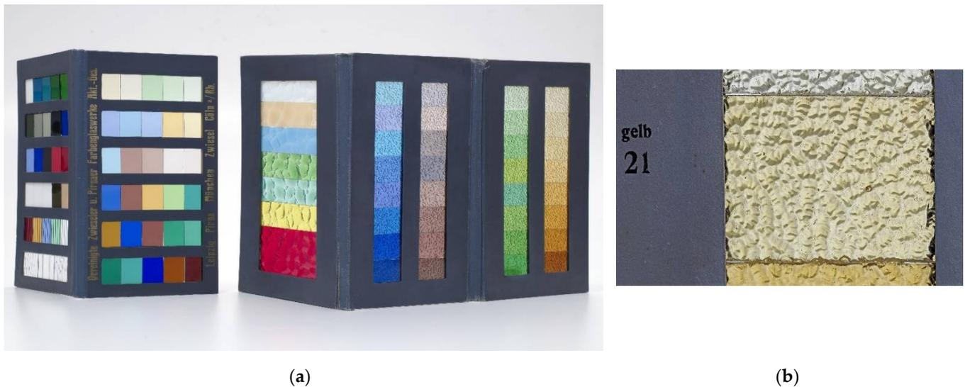
**Figure 17.** Template of the former glass manufacturer: (a) a whole range of colors and (b) ornamental glass in a yellowish color used during the renovation of Centennial Hall, in accordance with the original documentation.
