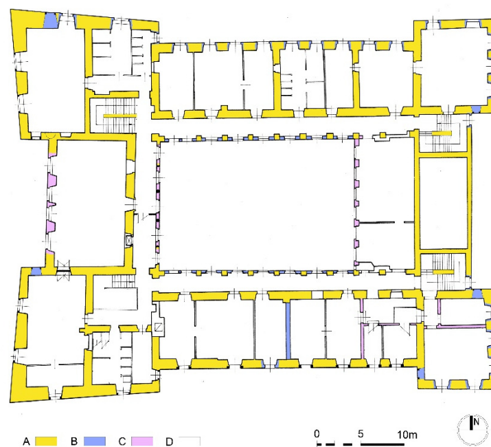
Figure 10. Prószków castle: second floor plan with chronological stratification of the walls. Legend: A—Renaissance (approximately 1563); B—Baroque (1667–1686); C—1881; D—walls unknown and from the 20th century, created by authors.
