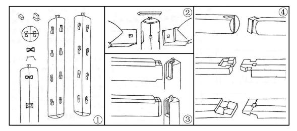
Figure 3. Schematic diagram of parts of tenon and mortise structure in Rules of Architecture.
