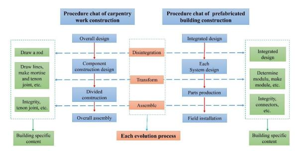
Figure 6. Procedure charts of carpentry work construction and prefabricated building construction.
