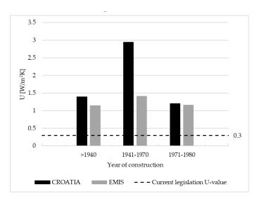
Figure 2. Characteristic U-values for external walls according to the year of construction.
