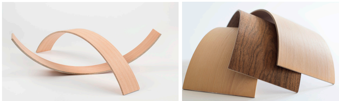
Figure 2. Double-sided veneering of flexible biocomposite defines a stable curved shape. © BioMat/ITKE—University of Stuttgart.
