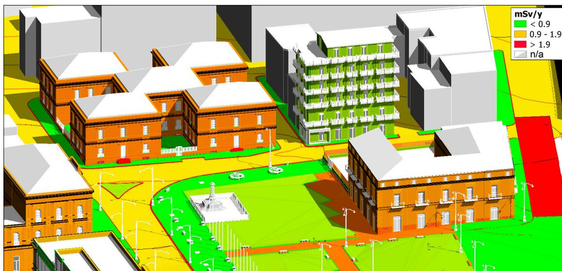
**Figure 3.** Pompei, Bartolo Longo Square. City Information Modelling (CIM) axonometric view, towards eastern side, categorized with Yearly Equivalent Dose proceeding from flooring and building materials.
