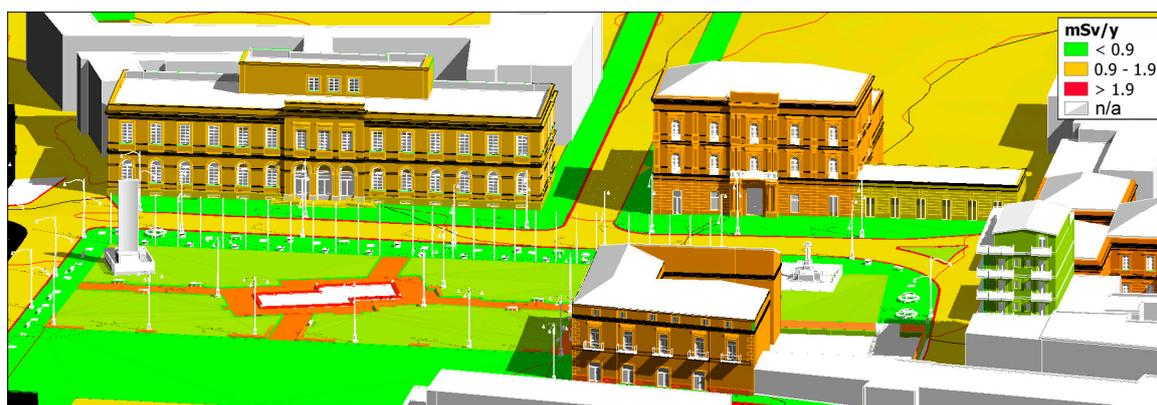
**Figure 4.** Pompei, Bartolo Longo Square. CIM axonometric view, towards south side, categorized with Yearly Equivalent Dose proceeding from flooring building materials.
