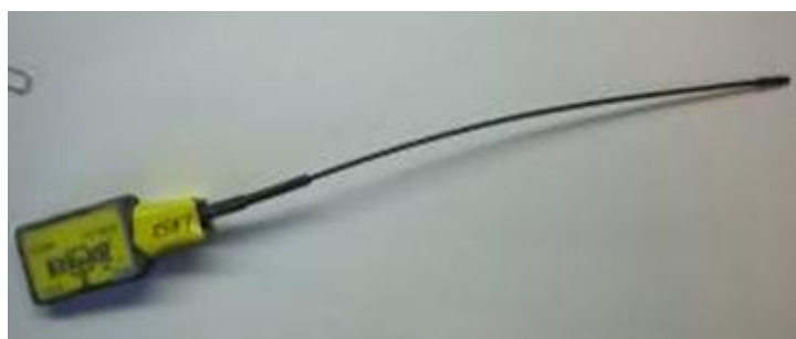
Figure 5. Very High Frequency (VHF) signal transmitter collar used in the positioning system.
