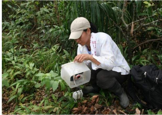
Figure 11. An automated photograph system with an infrared sensor.
