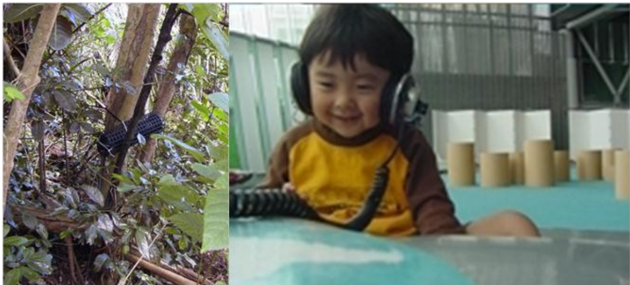
Figure 6. Live sound from a subtropical forest on Iriomote Island is collected via a pair of networked microphones that are wrapped in a thick black sheet of waterproof sponge and a plastic hard mesh, then tied to a tree trunk; such live sounds have been streamed to users in real time, 24 h a day since 1997. Photo (right) by SoundBum [6].
