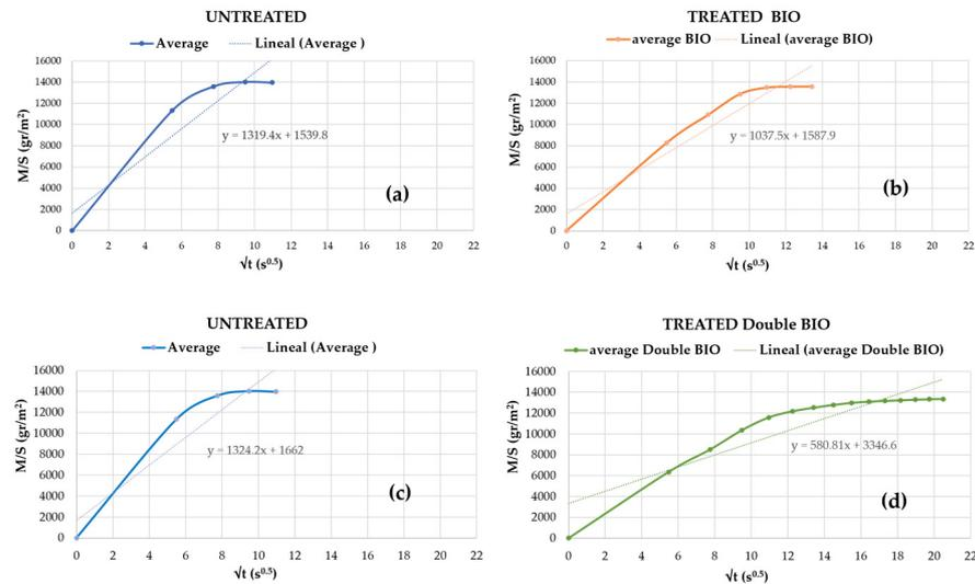
**Figure 10.** Capillary absorption graph at the same specimens (before and after being treated): (a) untreated specimens (before applying the bioconsolidant); (b) treated specimens with bioconsolidant; (c) untreated specimens (before applying the double bioconsolidant); (d) treated specimens with double bioconsolidant. Less capillary absorption is seen in the double-treated specimens.
