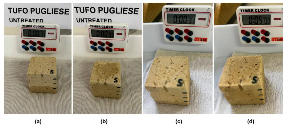
**Figure 11.** Photographs of the capillary absorption test of specimen 5. (a) Untreated at 11 s. (b) Untreated at 59 s. (c) Bioconsolidated with double treatment at 31 s. (d) Bioconsolidated with double treatment after 5 min.
