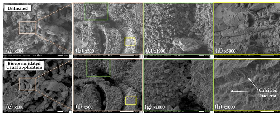
**Figure 8.** SEM observation of the same untreated and treated specimen. Colored frames indicate enlarged areas. The (top) row shows the untreated specimen, and the (bottom) row shows the bioconsolidated specimen with 7 days of treatment. The biofilm is visible in the last picture on the right.
