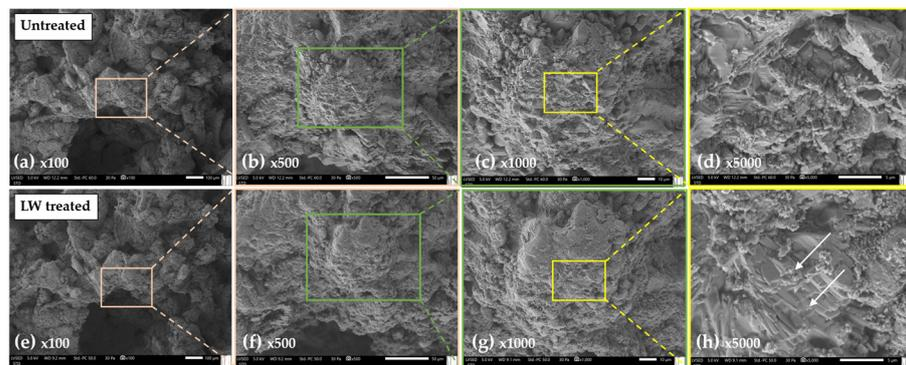
**Figure 12.** SEM observation of the same specimen untreated and treated with lime water. Colored frames indicate enlarged areas. The (top) row shows the untreated specimen and the (bottom) row the treated specimen. The arrows indicate the consolidated areas.
