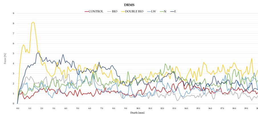
**Figure 18.** DRMS resistance graph. In the vertical axis, the resistance in N and in the horizontal axis, the depth of the test up to 200 mm.
