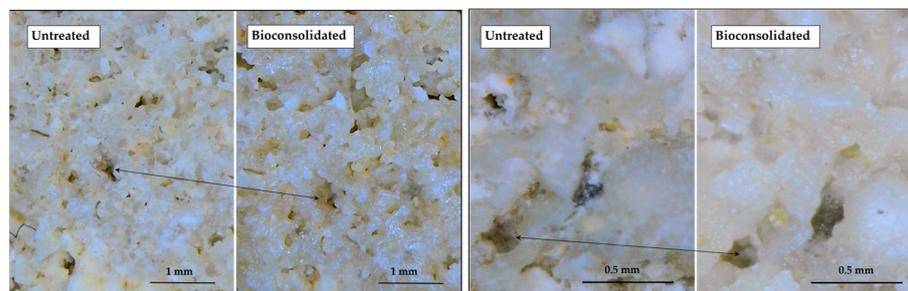
**Figure 7.** Handheld microscope view of the same specimen of Gravina Calcarenite, untreated and bioconsolidated with double application of the treatment. The orange areas correspond to the ankerite. The common zones are indicated in the images with the arrows.
