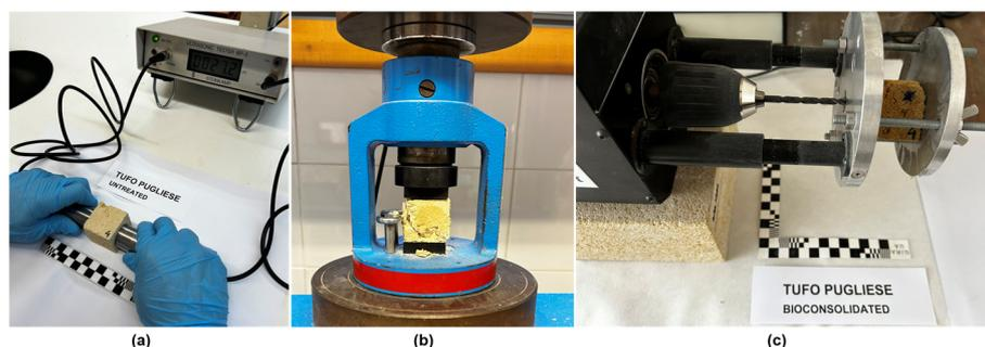
**Figure 5.** (a) Ultrasonic test. (b) Compression test. (c) DRMS testing process.
