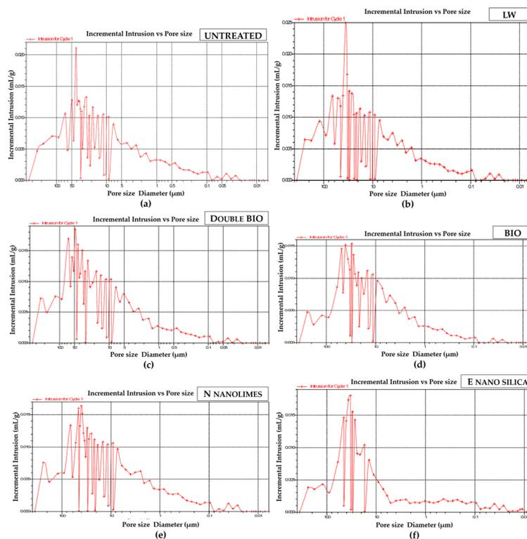
**Figure 19.** Pore size distribution graph. (a) Untreated. (b) Lime water. (c) Double bioconsolidation. (d) Bioconsolidation. (e) Nanolimes. (f) Nanosilica.
