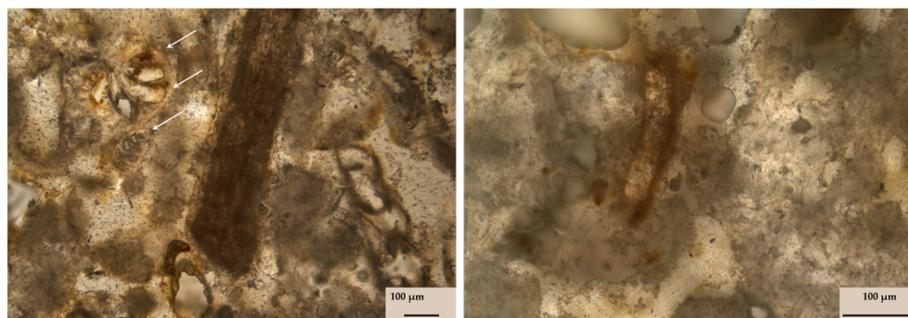
**Figure 3.** Thin-section micrographs of Gravina Calcarenite used in these studies. Marine fossils are marked with white arrows. It has been observed through a polarizing petrographic microscope.
