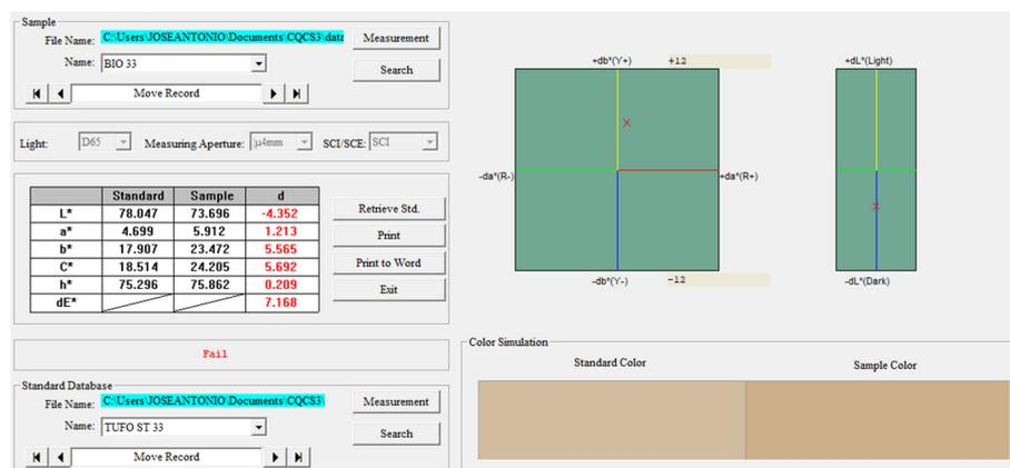
**Figure 6.** Colorimetric data of color difference between the same specimen (disk n° 3) untreated (standard) and treated with bioconsolidant for 7 days (sample). It can be seen that the total difference is  $\Delta E^* = 7.168$ , a value higher than 3, the limit at which it is invisible to the naked eye.
