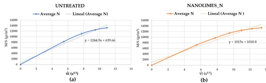
**Figure 15.** Capillary absorption graph of the same specimens: (a) untreated; (b) treated with nanolimes.
