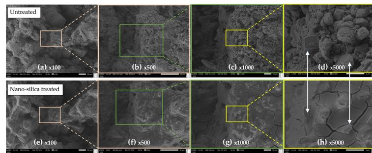
**Figure 16.** SEM observation of the same specimen untreated and treated with nanosilica (Nano Estel). In the (**upper**) row is the untreated specimen and in the (**lower**) row the treated specimen. Colored frames indicate enlarged areas. The arrows point to the same areas before and after being treated.
