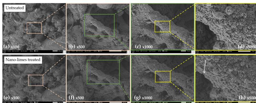
**Figure 14.** SEM observation of the same specimen untreated and treated with nanolimes. In the (upper) row is the untreated specimen and in the (lower) row the treated specimen. Colored frames indicate enlarged areas. The arrow indicates the consolidated areas.
