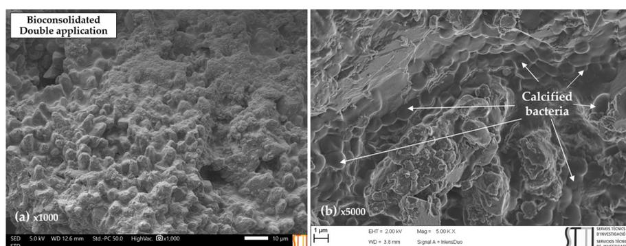
**Figure 9.** (a) SEM view of the specimen treated with double application of bioconsolidant showing at 1000 $\times$  magnification the entire surface enveloped by biofilm. (b) FE-SEM observation of Gravina Calcarenite with double bioconsolidant treatment. At 5000 magnification, the calcified bacteria can be distinguished with rounded shapes that surround and consolidate the original stone matrix.
