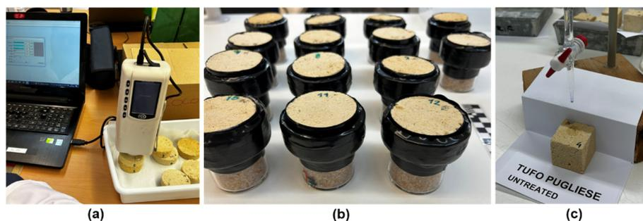
**Figure 4.** (a) Color study with colorimeter. (b) Glass containers with the specimens after water vapor permeability test. (c) Droplet absorption test.
