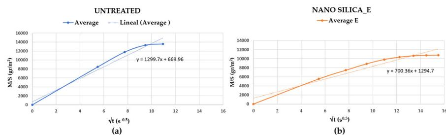
**Figure 17.** Capillary absorption graph of the same specimens: (a) untreated; (b) treated with nanolimes.
