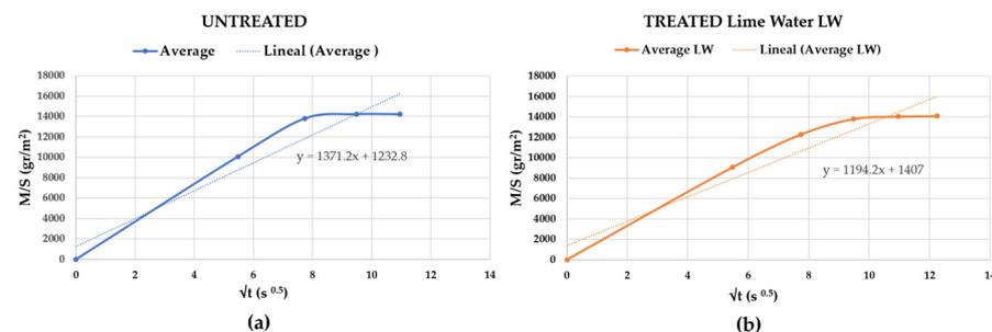
**Figure 13.** Capillary absorption graph of the average of the same specimens: (a) untreated; (b) treated with lime water.
