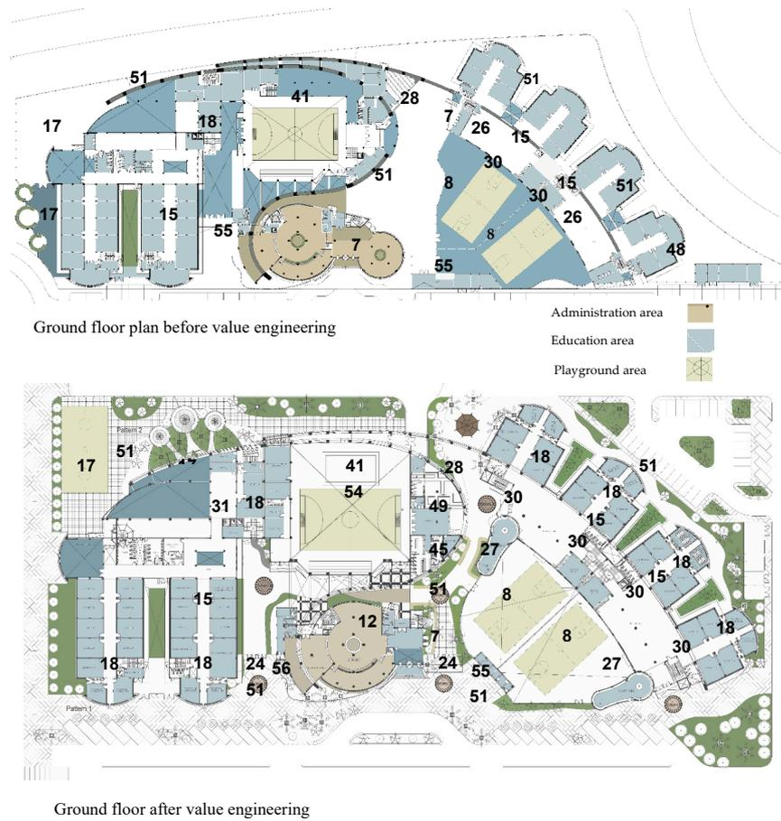
Figure 3. Applying value engineering ideas on the ground floor of the case study project.
