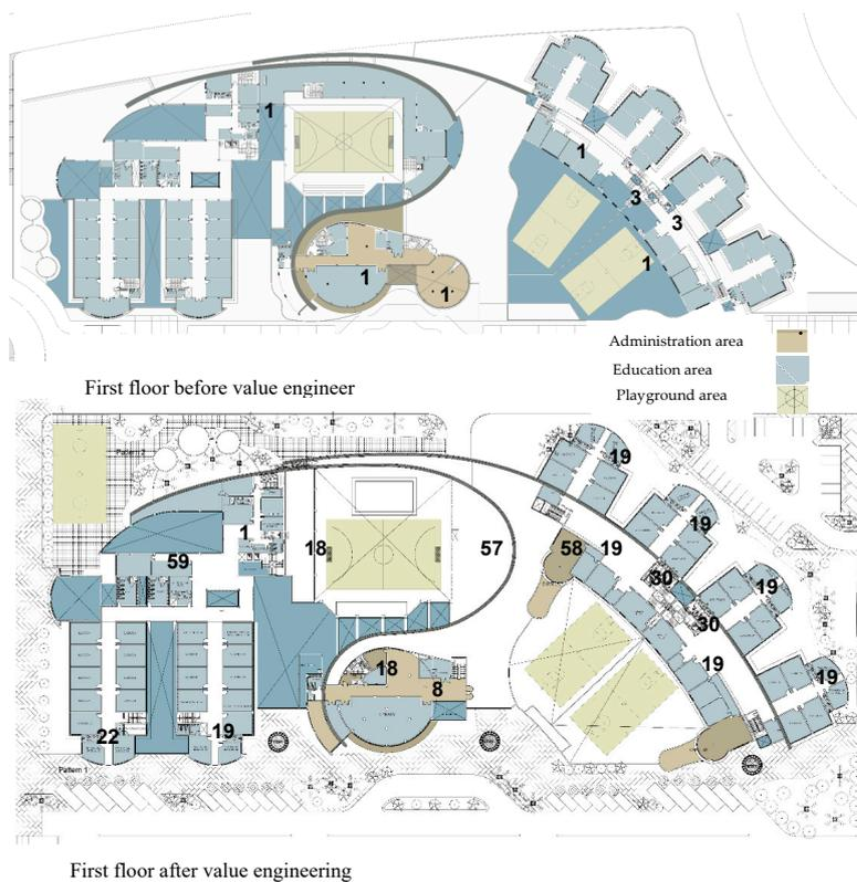
Figure 4. Applying value engineering ideas on the first floor of the case study project.
