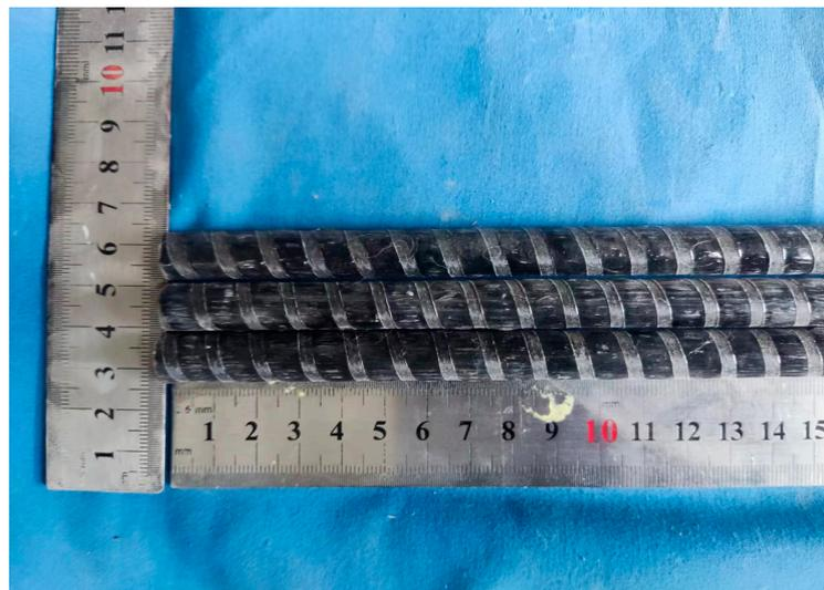
Figure 3. Steel-FRP composite bars.
