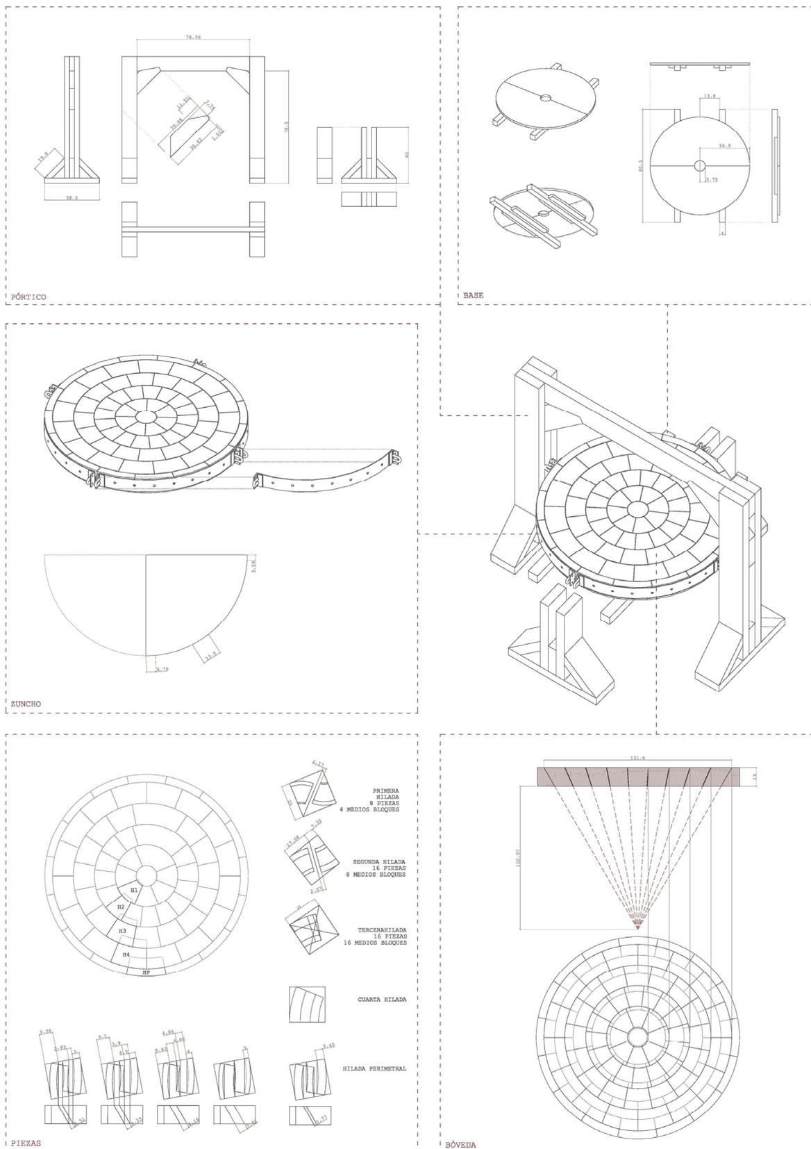
**Figure 16.** Graphics of reduced flat vault model tested at Stonework Workshop of the School of Architecture (Polytechnic University of Madrid), with lifting mechanism used (graph courtesy by Enrique Rabasa [15]).
