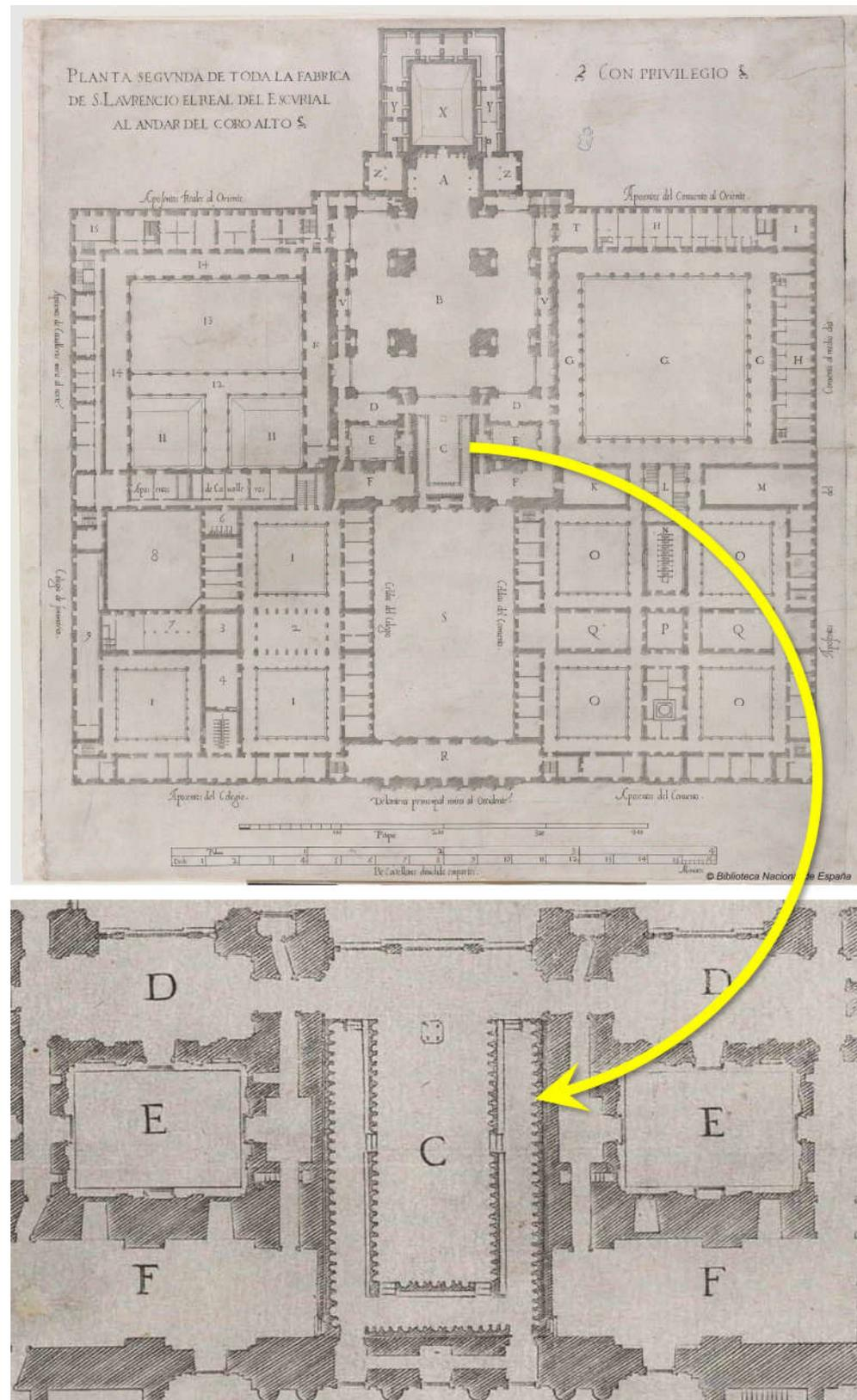
**Figure 4.** Plan of the same area of Basilica (Figure 3) at the level of the choir (first floor), with the position of the choir (C) over the flat vault (graphic by author from a plan by Juan de Herrera [4]).
