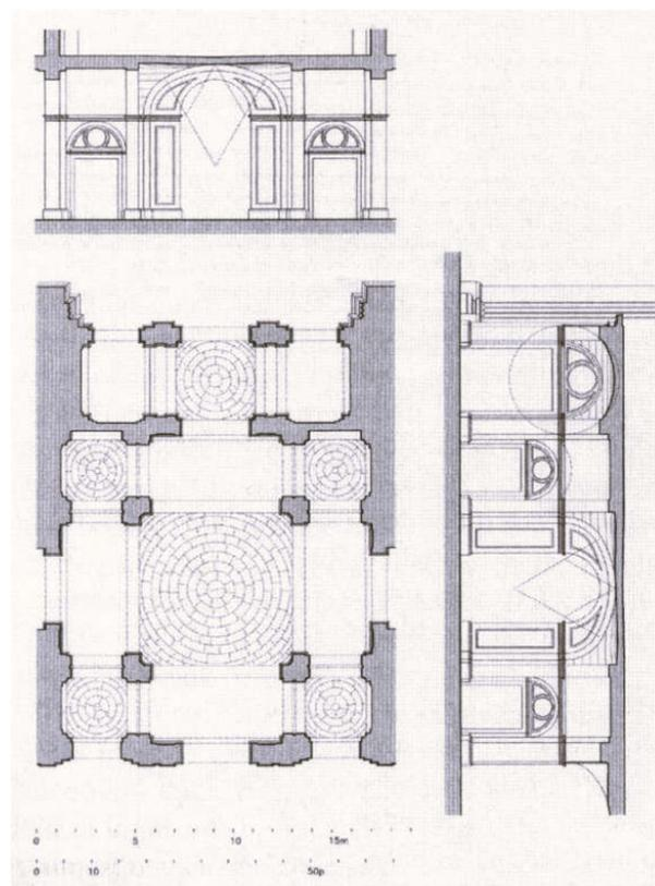
**Figure 8.** Plan and sections of narthex of the Basilica of El Escorial [8].
