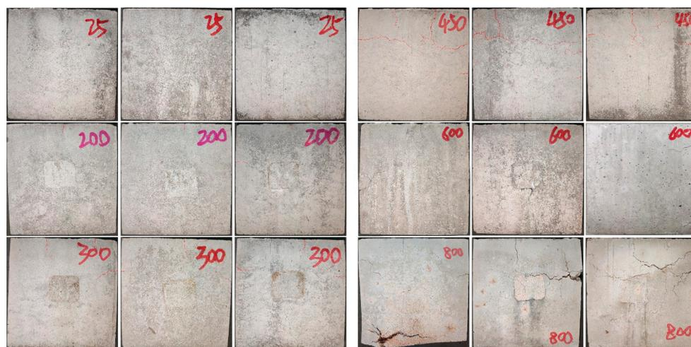
**Figure 9.** Appearance of the LZTRSC specimen exposed to elevated temperatures.
